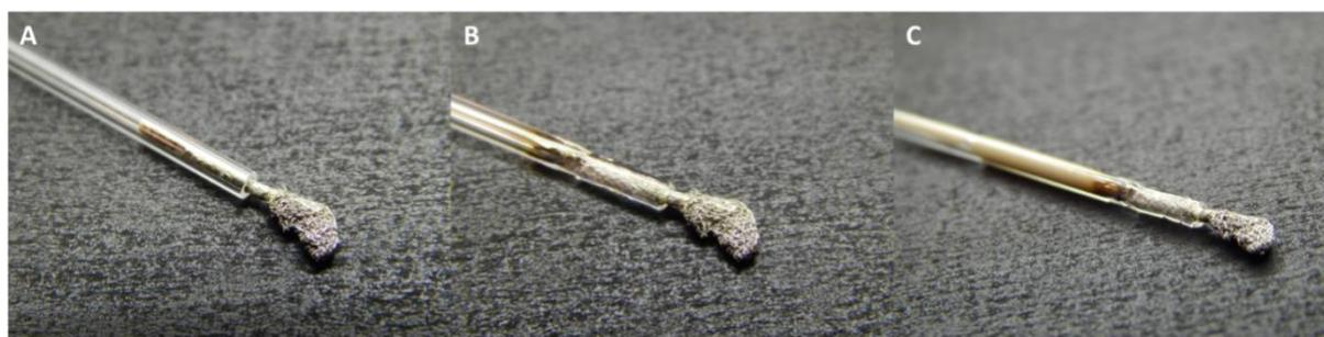
Figure 2.5: Successive steps of electrode preparation
