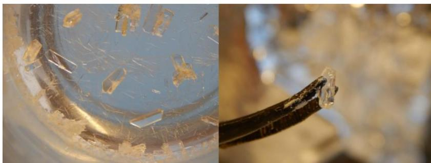
Figure 2.2: BTPPA<sup>+</sup>TPBCl<sup>-</sup> crystals after acetone evaporation
