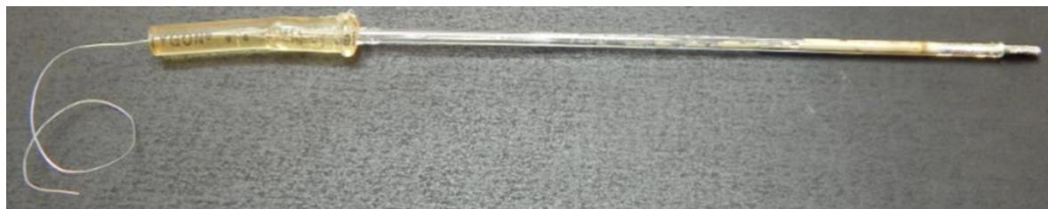
**Figure 2.6:** Platinum mesh based counter electrode
