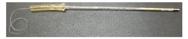
Figure 2.6: Platinum mesh based counter electrode
