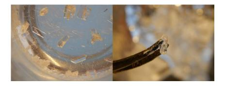
Figure 2.2: BTPPA+TPBCl- crystals after acetone evaporation
