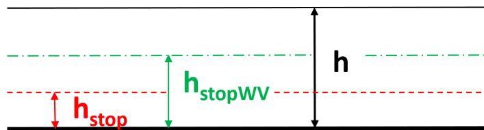
FIGURE 5.14 – Sketch of a three-layer flow. h , h_{stopWV} and h_{stop} are respectively the depth of the flow, the deposits without vibrations and the deposits with vibrations.
