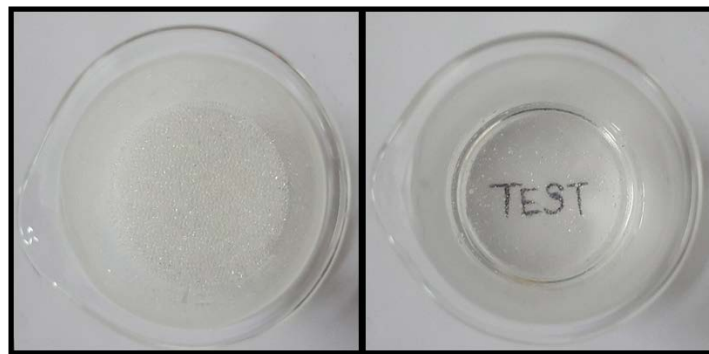
FIGURE 3.9 – Top view of the sample to test the readability of a text through 10 sizes of particles. The sample is made of borosilicate beads of d = 1 mm diameter in air ( left ), the refractive-index is matched with bidistilled glycerol ( right ) : media and fluid have optical indexes equal n_D = 1.473 .
