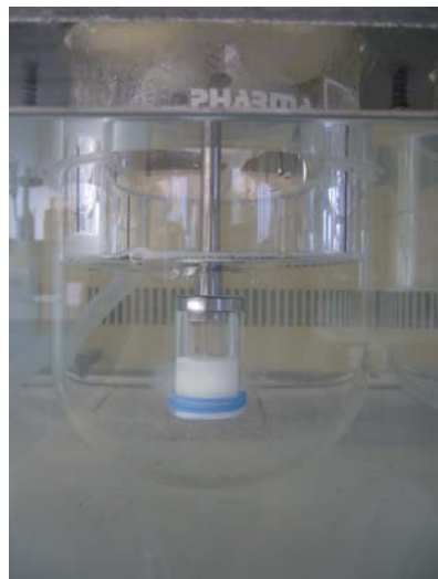
Figure 35: Nanosuspension located in the glass cell. Polymeric nanosuspension is separated from dissolution medium by a dialysis membrane (CE, 14000 kda, SpectraPor, Spectrum Labs, Breda, Netherlands).
