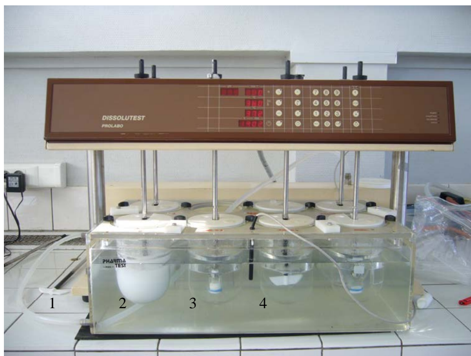
Figure 36: Two different techniques to perform the kinetic drug release. (1 and 3) represent direct dispersion of nanosuspension in the dissolution mediums, (2 and 4) represent the glass cells closed with dialysis membrane containing polymeric nanosuspension.
