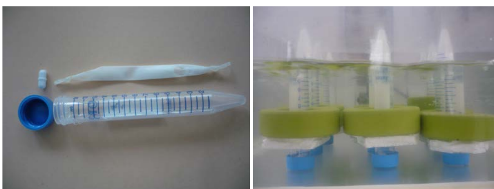
Figure 37: Dialysis bag method. Left picture shows the dialysis bag containing drug-loaded nanosuspension. Right picture shows the plastic tube containing the dialysis bag into a water bath.
