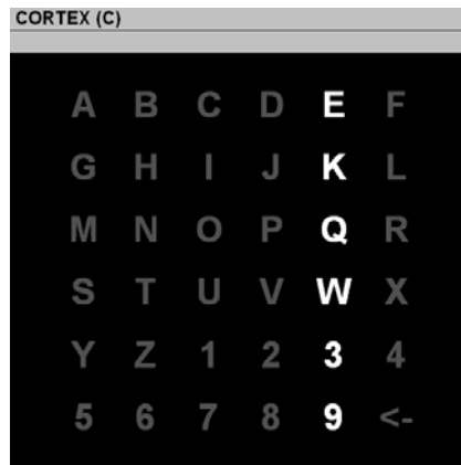
Figure 2.7: A 6x6 P300 speller. The application highlights in a random order columns and rows. The user looks at the desired letter. When the letter is highlighted, a P300 is generated. Detecting this specific transient event twice to identify the right column and the right row, it is possible to know which letter is requested.
