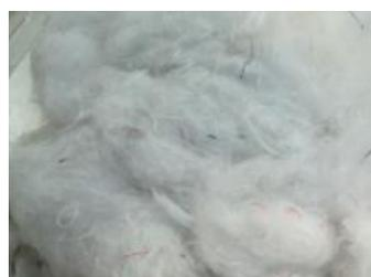
The coating of some airbags is not problematic for the opening process. Good results, well opened fibers, good length, good tensile strength. Harder material to treat. Plan at least 6 rolls. Limited production.
