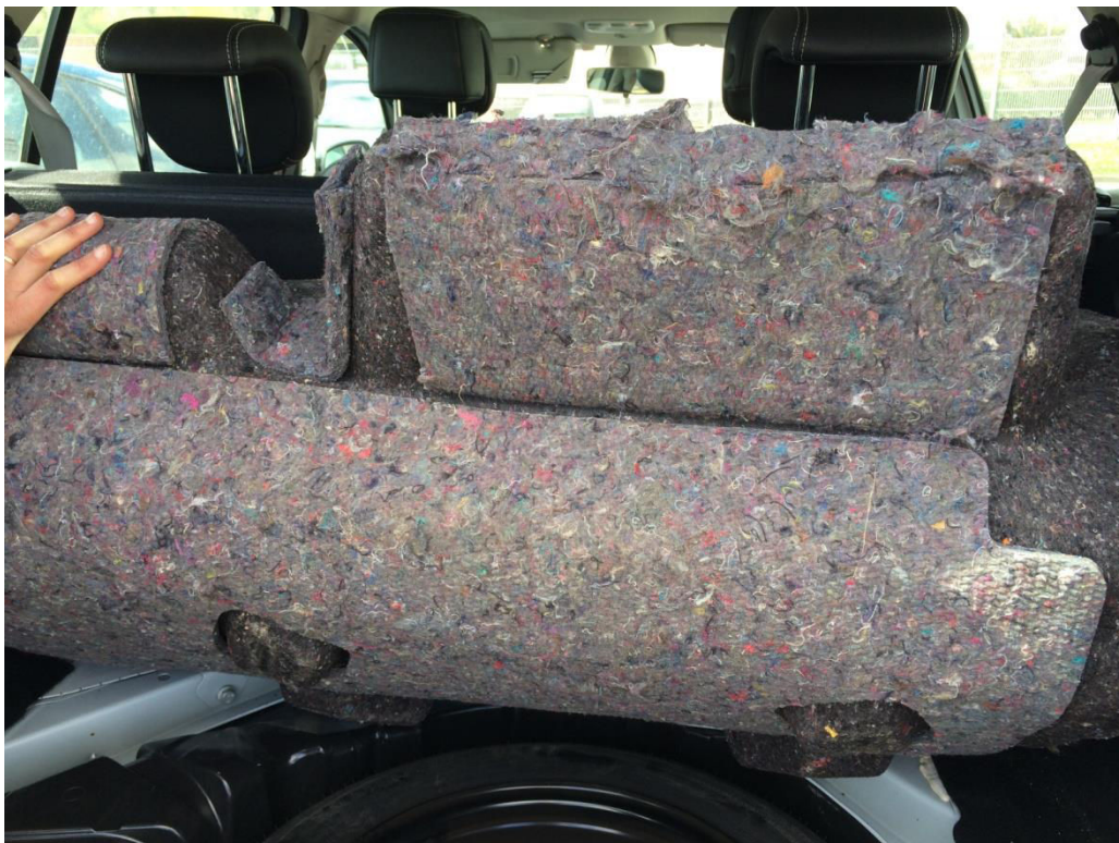
Figure 25 : A Photo of a Megan-Renault under-carpet trunk, a sound insulating application
