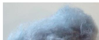
Very good results obtained with well opened fibers, good length and good tenacity. It requires 4 or 5 rolls for an industrial process. Care the cutting step, determining the results, because it's a monofilament product.
