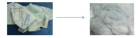
The coating of some airbags is not problematic for the opening process. Good results, well opened fibers, good length, good tensile strength. Harder material to treat. Plan at least 6 rolls. Limited production.
