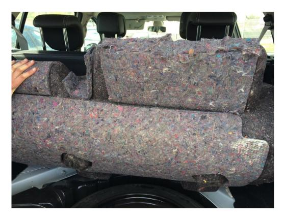
Figure 25 : A Photo of a Megan-Renault under-carpet trunk, a sound insulating application
