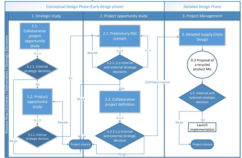
At different levels the details of the process are proposed. Especially for the 2<sup>nd</sup> stage, we present the details of the first step for a matter of understanding the organization between the activities. The
