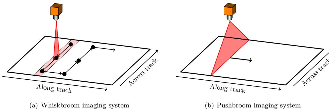
Figure 3.1: Data acquisition by hyperspectral imaging systems
