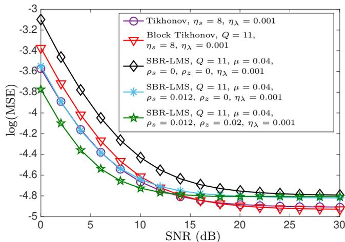
Figure 3.14: Performances of the hyperspectral image deconvolution algorithms
