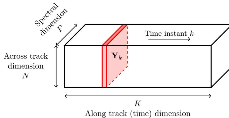
Figure 3.2: Structure of a hyperspectral data cube  $\mathbf{Y}$
