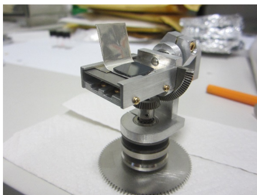
Fig. II-11: Experimental setup showing the sample holder for the sputter deposition of PS/PMMA on Ag foil
