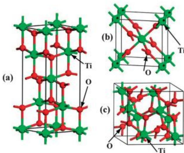
**Figure 2: Formes cristallines du  $\text{TiO}_2$  ; (a) anatase, (b) rutile, (c) brookite**
