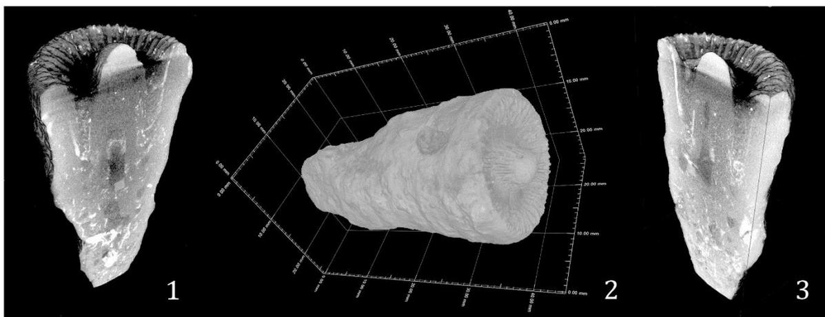
Figure 2: Examples of CT scan images provided by nanotom S phoenix 180 kV analysis on sample A57331-1. The slices through the coral presented in 1 and 3 are perpendicular to each other and
