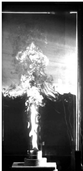
Figure 1: Image from experiment conducted in LEMTA laboratory showing the steady state of the simultaneous emptying-filling box process.
