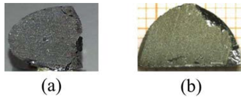
FIGURE 2.1: \text{Ba}_8\text{Au}_{5.25}\text{Ge}_{40.3}\square_{0.45} single crystal showing the faces perpendicular to (a) [100] and (b) [110] directions.
