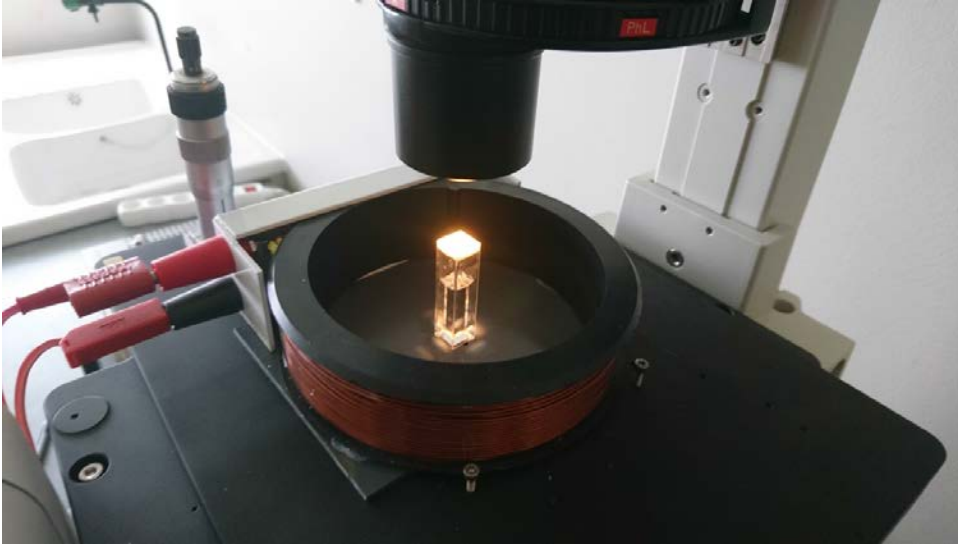
Figure 6.1: A picture of the experimental device with the coil centered around the rectangular recipient resting on a tilted plate.
