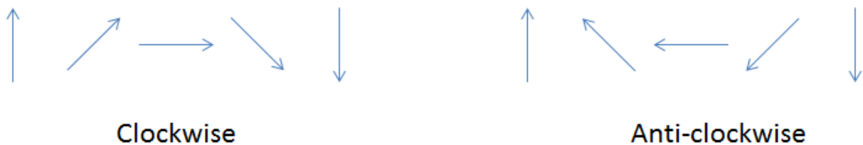
Figure I.5: Clockwise and anti-clockwise configurations for a Néel DW in a sample with an out of plane easy axis of magnetization. Each arrow represents a magnetic moment.
