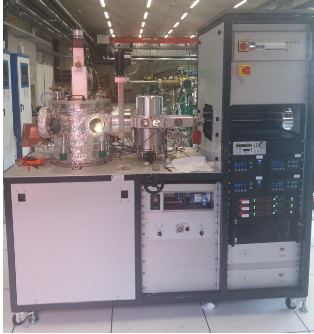
Figure II.2: Picture of the Vinci system used for deposition in IJL
