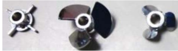
Figure 4.2: Impeller designs used for CFD simulations. Left to right: four-blade Rushton turbine, three-blade Elephant Ear impeller and three-blade marine propeller. Picture reproduced from Collignon et al. (2016) [1].
