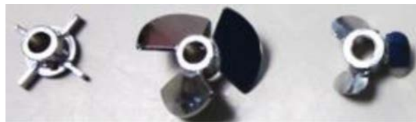
Figure 4.2: Impeller designs used for CFD simulations. Left to right: four-blade Rushton turbine, three-blade Elephant Ear impeller and three-blade marine propeller. Picture reproduced from Collignon et al. (2016) [1].
