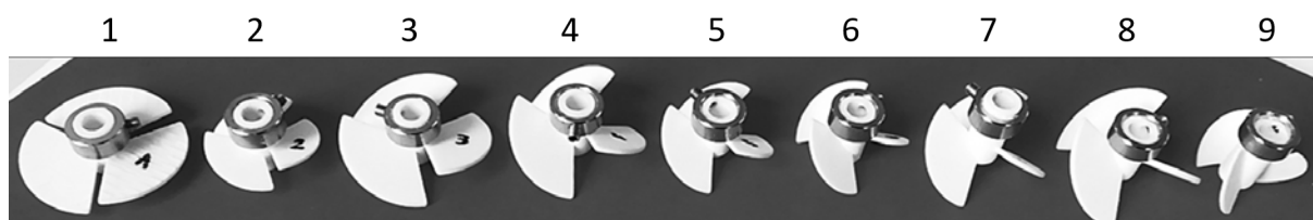
Figure 4.9: EE impellers built using 3D-printing for N_{js} experimental measurements.
