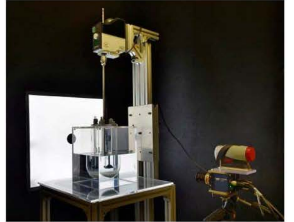
Fig. 4. Configuration of the experimental apparatus for light attenuation measurements.
