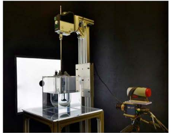
Fig. 4. Configuration of the experimental apparatus for light attenuation measurements.
