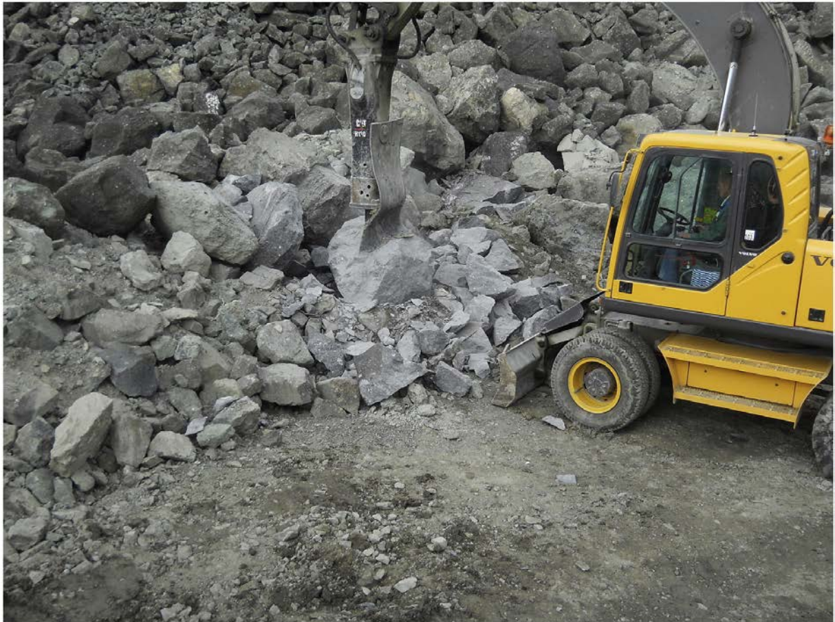
Photo of the mechanical rock breaker used to crush boulders of several tons.
