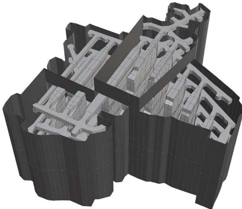
Fig. D.1 - Envelope (in black) built around galleries and stopes (in gray) for controlling mesh size within this area. Note that, for an easier visualization, the upper surface of the envelope has been intentionally removed from the image.
