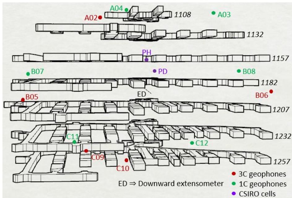
Fig. 2.11 - Geophysical and geotechnical monitoring network. Black numbers on the right refer to mine levels' depth.
