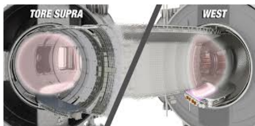
Figure 7.1: From the circular cross-section limiter Tore Supra to the D-shape cross-section divertor WEST (Tungsten (W) Environment in Steady-state Tokamak).
