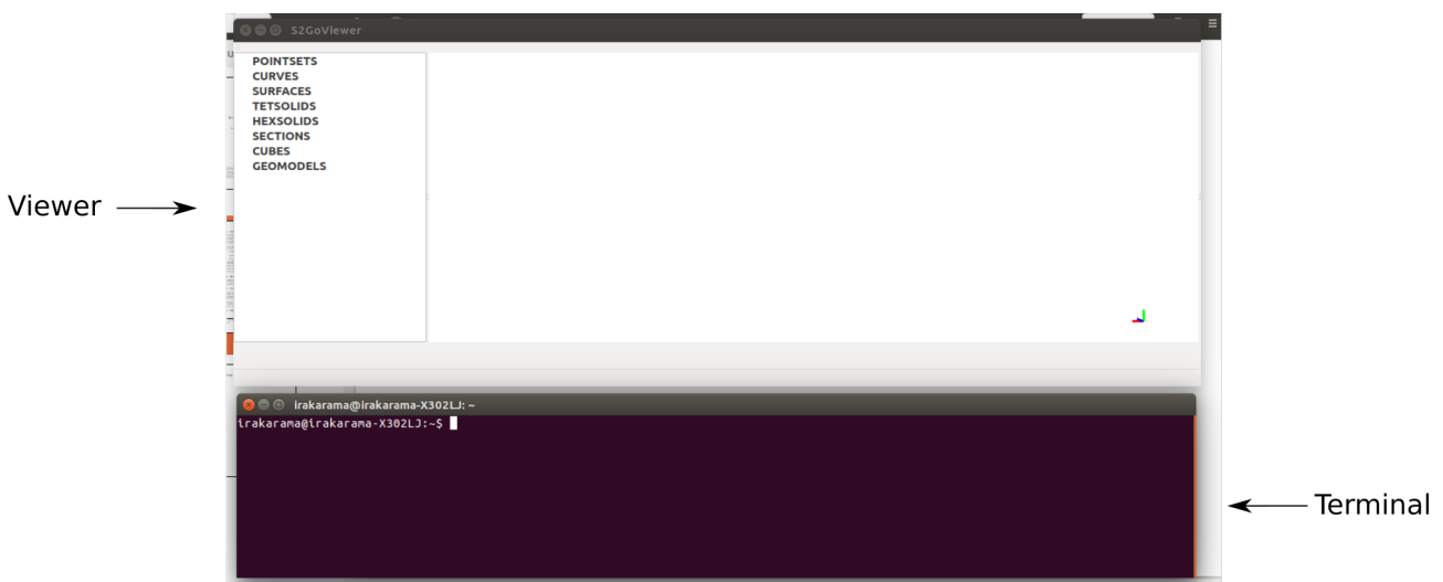
Figure 102: Getting started with SIGMA for the user. We launch the viewer, and then open a Linux terminal below it. The terminal is used not only to run stand-alone commands but also to interact with the viewer.
