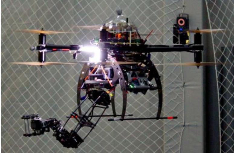
FIGURE 2.1: ARCAS multirotor with the attached 6-DoF manipulator [1].
