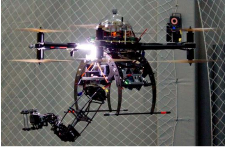
FIGURE 2.1: ARCAS multirotor with the attached 6-DoF manipulator [1].
