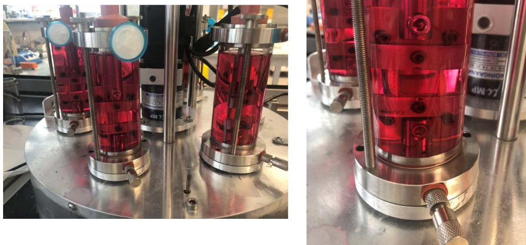
Figure 10 The tension-torsion bioreactor designed by our team.
