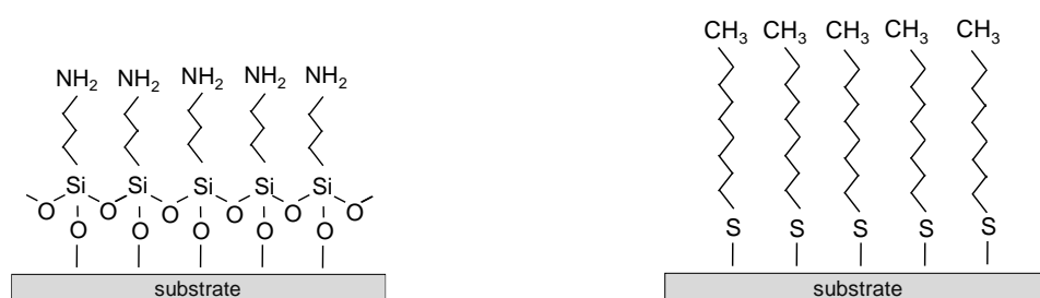
Figure 1.8. Schematic view of SAM supported on a substrate: a case of silanized surface on the example of (3-Aminopropyl)trimethoxysilane (left) and thiolated surface on the example of decanethiol (right)
