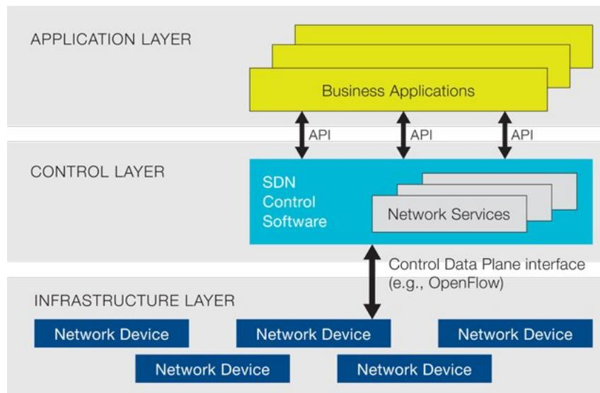
FIGURE 2.2 – Schéma de l'architecture SDN ([www.opennetworking.org](http://www.opennetworking.org))
