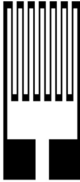
Figure 2.20 Schematic of the strain sensor gauge (Correia et al. , 2013)
