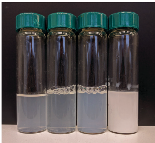
Figure 74: Mixed lanthanum chloride/sodium oleate solutions for the flotation tests that require a sodium oleate dosage of 100 \text{ g t}^{-1} and lanthanum dosages of 0/0.1/1/10 \text{ g t}^{-1} (from left to right)
