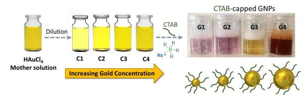
Scheme 12 Schematic representation of the synthesis of the CTAB-capped gold nanoparticles of different sizes using 5x10<sup>-5</sup> M, 8x10<sup>-5</sup> M, 10<sup>-3</sup> M and 10<sup>-2</sup> M of gold precursor concentration for G1, G2, G3 and G4 respectively.
