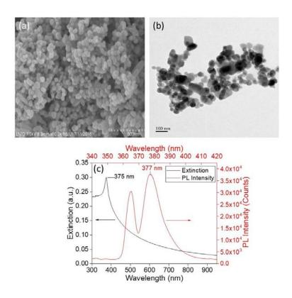
Figure 29 ZnO NPs annealed at 250°C (a) SEM-FEG image and (b) TEM image and (c) extinction (black) and average photoluminescence (red) of three PL spectrum measured separately (laser power is slightly different).
