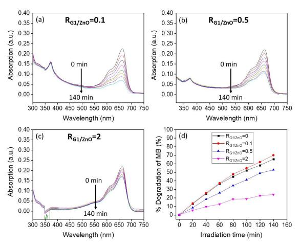
Figure 37 Absorption of G1-loaded ZnO ( $T_{ann}$ =250°C)-MB mixture with UV irradiation for different irradiation time intervals lasting for 140 min at different GNPs/ZnO ratios (a)  $R_{G1/ZnO}$ =0.1, (b)  $R_{G1/ZnO}$ =0.5, (c)  $R_{G1/ZnO}$ =2, (d) % degradation of MB using the three ratios G1/ZnO mixed with MB as a function of irradiation time.
