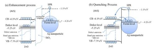
Scheme 2 A schematic diagram showing the PL enhancement (a) and quenching (b) processes. Adapted from ref. [197].
