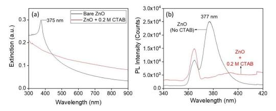
Figure 53 ZnO NPs before and after the addition of 0.2 M CTAB solution (a) extinction spectrum and (b) UV zone of the photoluminescence spectrum.
