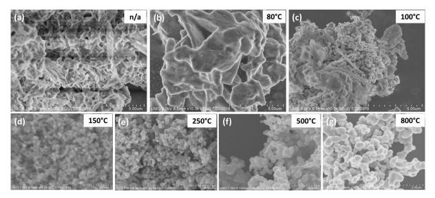
Figure 21 SEM images of the synthesized ZnO NCs: (a) before annealing (n/a), annealed at (b-g) 80, 100, 150, 250, 500 and 800 $^{\circ}$ C, respectively. The scale bar in images (a-c) is 5  $\mu$ m, (d-f) 500 nm, and (g) 2  $\mu$ m.
