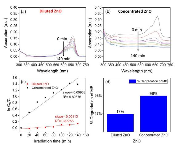
Figure 36 Absorption of ZnO ( $T_{ann}$ =250°C)-MB mixture with UV irradiation for different irradiation time intervals lasting for 140 min using (a) diluted solution of ZnO catalyst, and (b) concentrated solution of the same ZnO catalyst, (c) the variation of  $InC_0/C$  of both catalysts concentrations with irradiation time lasting for 140 min, (d) % degradation of MB by different concentrations of ZnO catalyst.
