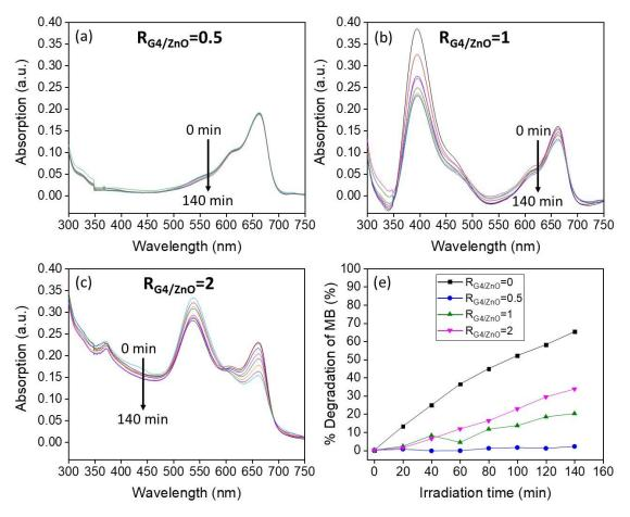
Figure 40 Absorption of G4-loaded ZnO ( $T_{ann}$ =250°C)-MB mixture with UV irradiation for different irradiation time intervals lasting for 140 min at different GNPs/ZnO ratios (a)  $R_{G4/ZnO}$ =0.5, (b)  $R_{G4/ZnO}$ =1, (c)  $R_{G4/ZnO}$ =2, (d) % degradation of MB using the three ratios G4/ZnO mixed with MB as a function of irradiation time.
