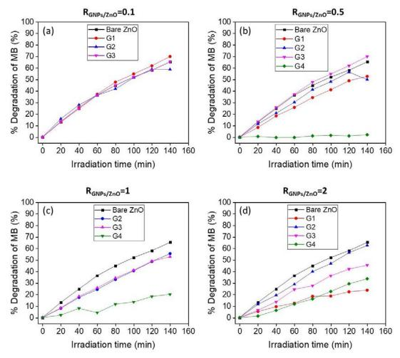
Figure 41 % degradation of MB using GNPs/ZnO catalyst in different sizes at (a)  $R_{GNPS/ZnO}$ =0.1, (b)  $R_{GNPS/ZnO}$ =0.5, (c)  $R_{GNPS/ZnO}$ =1, (d)  $R_{GNPS/ZnO}$ =2.
