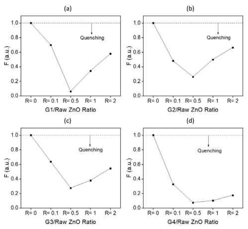
Figure 52 UV-PL modification factor of the raw material synthesis ZnO NPs annealed at  $150^{\circ}$ C upon coupling with different ratios  $R_{GNPs/raw\ ZnO} = 0.1$ , 0.5, 1 and 2 into CTAB-capped gold nanoparticles; (a) G1, (b) G2, (c) G3 and (d) G4.
