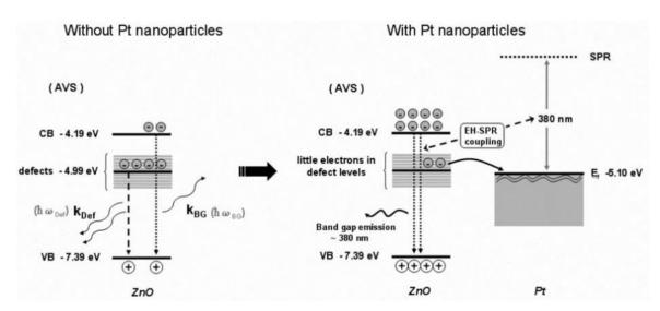
Scheme 3 A schematic diagram for the coupling between bandgap and surface plasmon resonance, and carriers transfer between the defect level and the Pt Fermi level. It results in enhanced bandgap emission and suppressed defect emission. Adapted from ref. [199].
