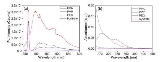
Figure 56 Different stabilizers as PVA, PVP, PEG, K<sub>3</sub>citrate (2 mg) dissolved in 2 ml water (a) Room temperature PL spectra, (b) UV-Vis absorption spectra.
