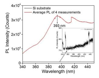
Figure 47 Room temperature average photoluminescence spectrum of ZnO NPs embedded PMMA nanolayer over Si substrate taken at four different positions. The inset corresponds to the PL measurements of the silicon (Si) substrate as a reference.
