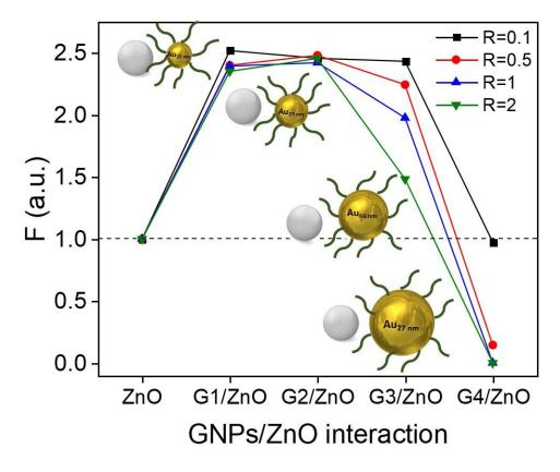
Figure 34 UV-PL modification factor of ZnO NPs solutions before and after the addition of increased sizes GNPs G1, G2, G3, and G4 for all GNPs/ZnO ratios.
