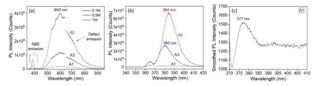
Figure 15 Photoluminescence measurements of different samples of ZnO QDs solutions (A1, A2 and A3) after annealing at 150°C (a) the full PL spectrum showing break line at the missing data points over the region of the second order of the laser. (b) ZnO UV region of the PL spectrum, (c) zoom in the UV-region of the smoothed PL spectrum of the solution A1 (0.1 M raw materials).
