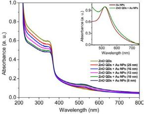
Figure 7 Absorption spectra of ZnO QDs (16.7  $\mu$ M) in the absence and presence of Au NP (0.67  $\mu$ M) of five different sizes. The inset shows the change in the surface plasmon band of Au NP upon interaction with the ZnO QDs. Adapted from ref. [163].
