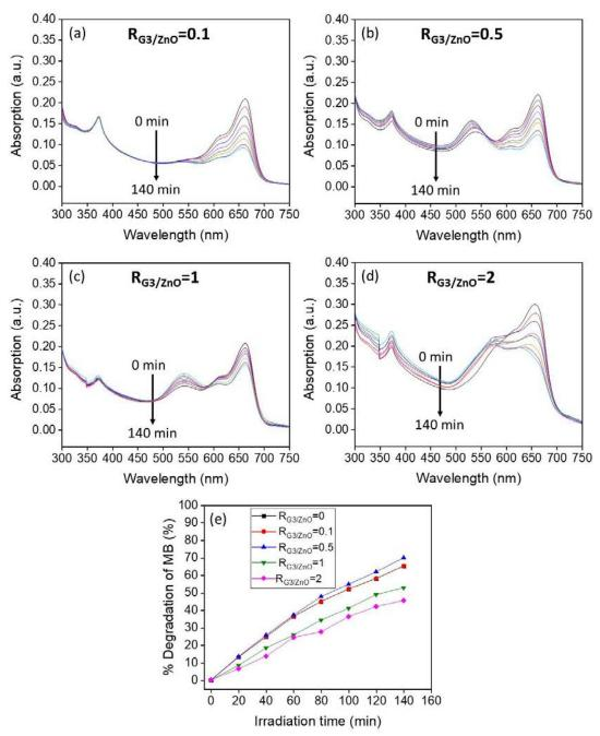
Figure 39 Absorption of G3-loaded ZnO ( $T_{ann}$ =250°C)-MB mixture with UV irradiation for different irradiation time intervals lasting for 140 min at different GNPs/ZnO ratios (a)  $R_{G3/ZnO}$ =0.1, (b)  $R_{G3/ZnO}$ =0.5, (c)  $R_{G3/ZnO}$ =1, (d)  $R_{G3/ZnO}$ =2, (e) % degradation of MB using the four ratios G3/ZnO mixed with MB as a function of irradiation time.
