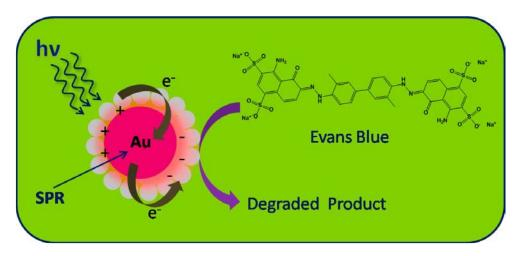
Scheme 8 Schematic Presentation of the Photocatalytic Degradation of Evans Blue at the ZnO-Au Hybrids Surfaces. Adapted from ref. [163].
