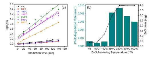
Figure 27 (a)  $1^{st}$  order equation of the kinetic reaction of different sizes of ZnO NPs annealed at different temperatures plotted by  $ln(C_0/C)$  versus irradiation time and (b) comparative photodegradation rates of MB dye with different sizes of ZnO NPs annealed at various temperatures.
