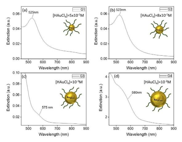
Figure 31 Extinction spectra of the CTAB-capped gold nanoparticles produced using 0.2 M of CTAB as a capping agent (a) G1 of  $[HAuCl_4]=5x10^{-5} M$ , (b) G2 of  $[HAuCl_4]=8x10^{-5} M$ , (c) G3 of  $[HAuCl_4]=10^{-3} M$ , (d) G4 of  $[HAuCl_4]=10^{-2} M$  (smoothed curve).
