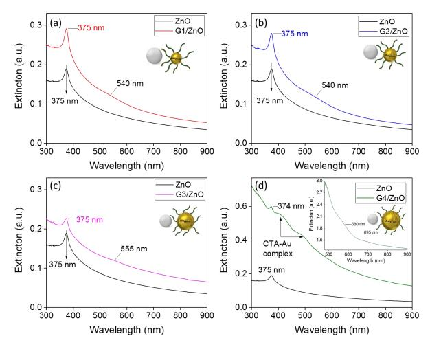
Figure 32 Extinction spectra of ZnO NPs solution before and after the addition of GNPs (a) G1 ( $R_{G1/ZnO}$ =2), (b) G2 ( $R_{G2/ZnO}$ =2), (c) G3 ( $R_{G3/ZnO}$ =2), (g) G4 ( $R_{G4/ZnO}$ =0.1), the inset in (d) is the zoom in UV region of the extinction spectrum of coupling G4 to ZnO NPs in a ratio  $R_{G4/ZnO}$ =2.
