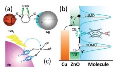
Scheme 4 The CT pathways in semiconductor-metal heterostructures (a) semiconductor-to-molecule-to-metal, (b) metal-to-semiconductor-to molecule, (c) metal-to-molecule-to-semiconductor. Adapted from ref. [213].
