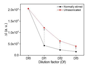
Figure 49 The variation of UV-PL intensity height ( $\Delta I$ ) as a function of increasing dilution factors Df1, Df2, Df3 corresponding to addition of 0.1, 1 and 2 ml of D.I. water to the clear dispersion solution representing Df0 as a reference. The black squared line represents the variation of  $\Delta I$  of the diluted solutions that were normally stirred,
