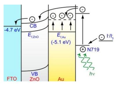
Figure 13 Energy-band diagram depicting the possible electron-transfer path in the ZnO/Au-hybrid DSSC, showing the Schottky barrier formed at the ZnO/Au interface. The dashed line in Au represents the position of the Fermi level of gold after electron injection from dye N719. Adapted from ref. [80].
