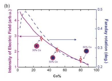
Figure 2 Calculated intensity of the electric field within the Co core in Co-Ag core-shell nanoparticles at resonance (continuous violet line) and maximum Faraday rotation of Co-Ag nanoparticles embedded in oil (n=1.5018) (dashed blue line) as a function of the Co concentration. Calculations show an excellent agreement with the experimental measurements (red dots). The error bars represent the standard error calculated by taking multiple measurements. Adapted from ref. [11].
