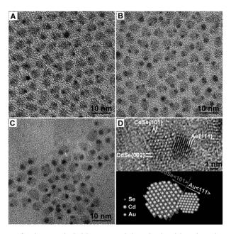
Figure 3 (A-C) TEM images of CdSe-Au hybrid nanoparticles obtained by changing QAu from 2, 4 to 6 µmol, respectively. The nanoparticles are seen as dimeric units, all with a similar size of ~3.4 nm for the CdSe component. (D) High-resolution TEM image and a schematic drawing of the CdSe-Au hybrid nanoparticles. Adapted from ref. [9].
