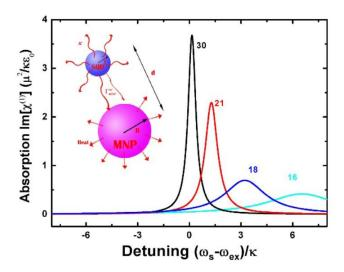
Figure 5 The signal light absorption spectrum of SQDs. The signal light absorption spectrum of SQDs for different distance d. The inset shows a complex system composed of a SQDs to a MNPs. A SQDs with radius r is placed in the vicinity of a MNPs with radius R. The center-to-center distance is d. Adapted from ref. [160].
