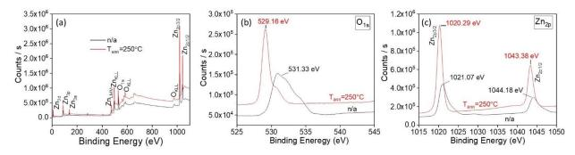
Figure 20 (a) XPS measurements of the synthesized ZnO NCs before (black curve) and after annealing at 250°C (red curve), (b) O<sub>1s</sub> spectrum, (c) Zn<sub>2p</sub> spectrum.
