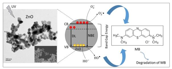
Scheme 10 Schematic representation of the photocatalytic activity of the ZnO NPs by degradation of methylene blue (MB) dye. (The photoluminescence of ZnO NPs is also indicated). The TEM image corresponds to the synthesized ZnO NPs annealed at 250°C. The inset in the TEM image is the SEM image of the same sample.
