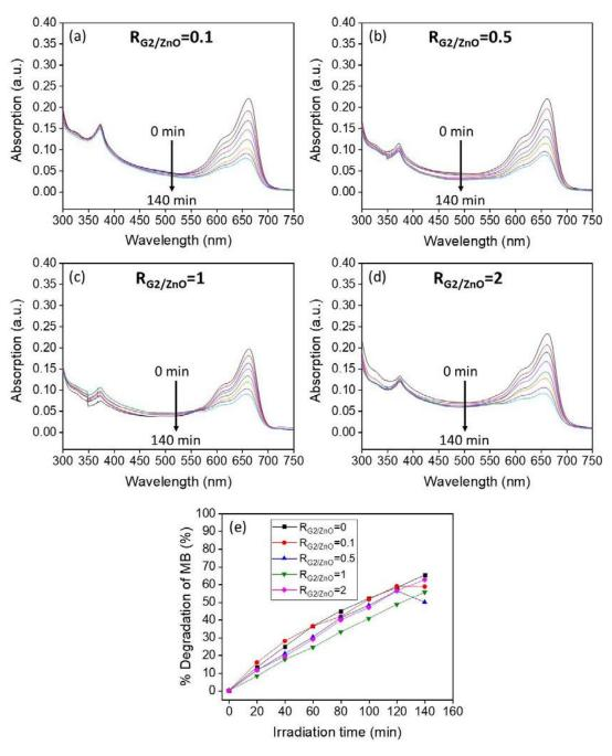
Figure 38 Absorption of G2-loaded ZnO ( $T_{ann}=250^{\circ}C$ )-MB mixture with UV irradiation for different irradiation time intervals lasting for 140 min at different GNPs/ZnO ratios (a)  $R_{G2/ZnO}=0.1$ , (b)  $R_{G2/ZnO}=0.5$ , (c)  $R_{G2/ZnO}=1$ , (d)  $R_{G2/ZnO}=2$ , (e) % degradation of MB using the four ratios G2/ZnO mixed with MB as a function of irradiation time.
