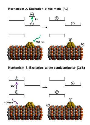
Figure 11 Two charge separation mechanisms in these hybrid heterostructures. Mechanism A starts by excitation at the metal at 532 nm, thus forming hot electrons (e<sup>-</sup>) and holes (h<sup>+</sup>) in the metal. The hot electrons are then transferred to the semiconductor's conduction band. Mechanism B starts with excitation at the semiconductor at 405 nm, thus forming electron–hole pairs at the semiconductor. Photogenerated electrons are then trapped by the gold. Adapted from ref. [162].
