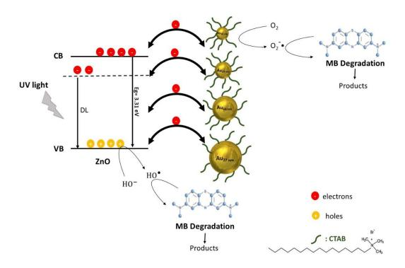
Scheme 14 Schematic representation of the charge transfer and the photocatalytic activity of CTAB-capped gold nanoparticles of different sizes loaded into ZnO NPs (DL: defect luminescence).
