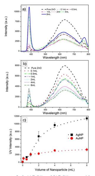
Figure 8 Photoluminescence spectra for the (a) ZnO/Ag and (b) ZnO/Au nanoparticles under excitation at 325 nm. (c) The ZnO UV-band intensity increases with increasing the metal nanoparticle concentration. Error bars represent the standard deviation for three separate measurements. Adapted from ref. [179].
