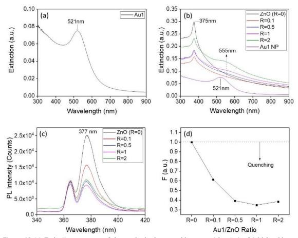
Figure 45 (a) Extinction spectrum of the synthesized pure gold nanoparticles Au1 of initial gold precursor concentration [HAuCl<sub>4</sub>]= 5x10<sup>-5</sup> M, hybrids after loading the ZnO NPs with different densities of pure GNPs (Au1) to have consecutive ratios of R=0.1, 0.5, 1 and 2 (R=0 represents the bare ZnO NPs without any addition of GNPs) (b) Extinction spectra, (c) UV-zone of the photoluminescence spectra and (d) UV-PL modification factor.
