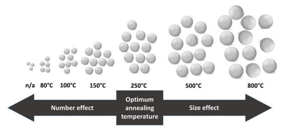
Scheme 11 Schematic representation of the ZnO nanocrystals with annealing temperatures showing the size and number effect on the photocatalytic activity. The gray spheres represents the ZnO NCs.
