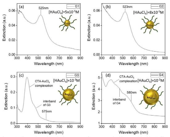
Figure 51 Full range (UV-Vis) extinction spectrum of CTAB-capped gold nanoparticles (a) G1 of [HAuCl<sub>4</sub>]=  $5x10^{-5}$  M, (b) G2 of [HAuCl<sub>4</sub>]=  $8x10^{-5}$  M, (c) G3 of [HAuCl<sub>4</sub>]=  $10^{-3}$  M, (d) G4 of [HAuCl<sub>4</sub>]=  $10^{-2}$  M. The inset in each spectrum illustrates the CTAB (green lines)-capped GNPs (golden spheres).
