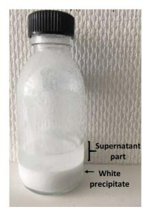
Figure 14 Image of the solution A3 after post-thermal treatment solution of as-synthesized QDs showing the two separated gradations: the transparent supernatant phase and the bottom white precipitate.
