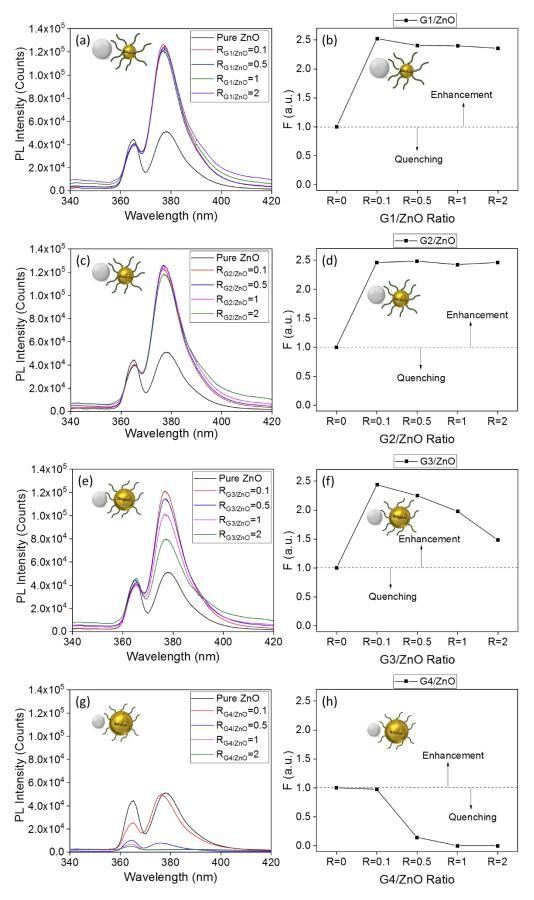
Figure 33 UV-zone of the PL spectra (right), and the UV-PL modification factor (left) of ZnO NPs solutions before and after the addition of (a,b) G1, (c,d) G2, (e,f) G3, and (g,h) G4.
