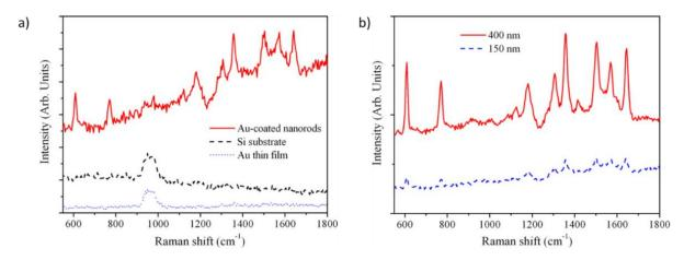
Figure 9 a) SERS spectra from Au-coated ZnO nanorods of 150 nm in diameter, Au thin film (5 nm thick), and a bare Si substrate with R6G of  $1\mu M$ . b) Comparison of SERS spectra of Au-coated ZnO nanorods of diameter of 400 and 150 nm with R6G of  $1\mu M$ . Adapted from ref. [212].
