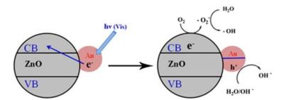
Scheme 6 Proposed mechanism of the photocatalysis of Au/ZnO nanostructures upon excitation of the visible light. Adapted from ref. [65].
