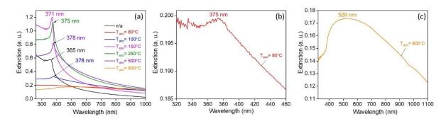
Figure 23 (a) UV-Vis absorption spectroscopy of the as-prepared non-annealed (n/a) ZnO NPs and after annealing at different temperatures, (b) zoom in the UV region of the ZnO nanocrystals annealed at 80°C, and (c) magnification of the UV-Vis absorption spectra of the ZnO nanocrystals annealed at 800°C.
