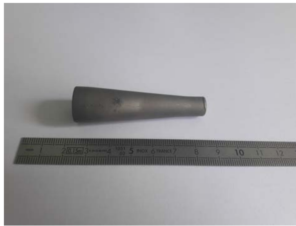
FIGURE 2.1 – Lingot tronconique en IN738LC
