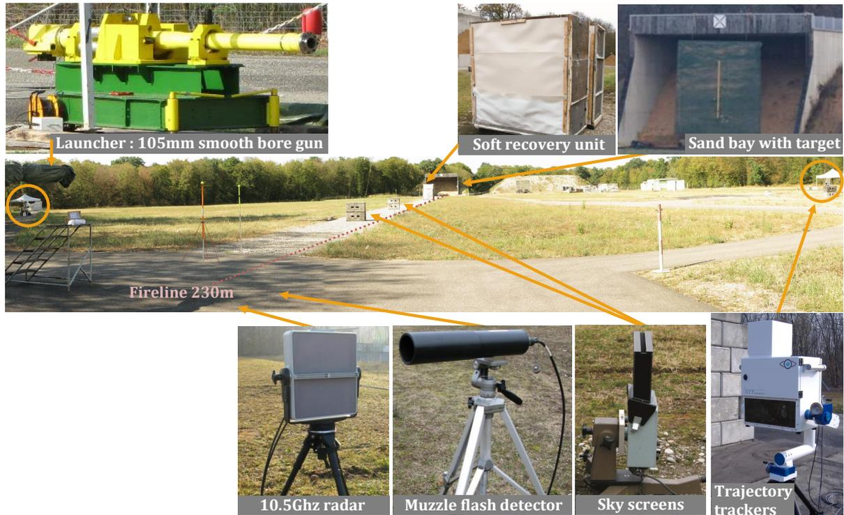
Figure 1.2: Example of experimental set-up on the ISL's test site.
