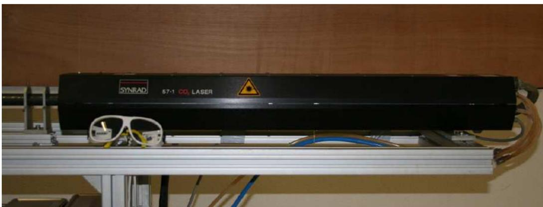
FIGURE 3.6 – Laser CO<sub>2</sub> SYNRAD 57-1 130 W [109]
