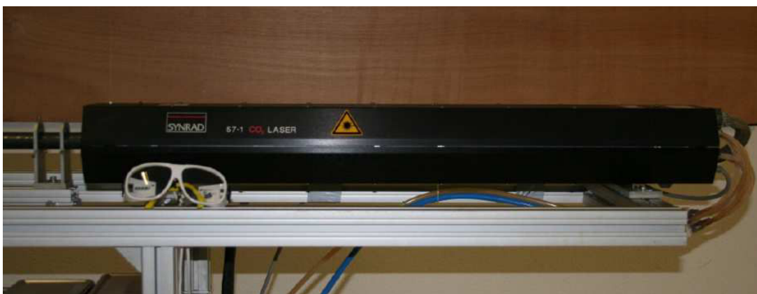
FIGURE 3.6 – Laser CO 2 SYNRAD 57-1 130 W [109]
