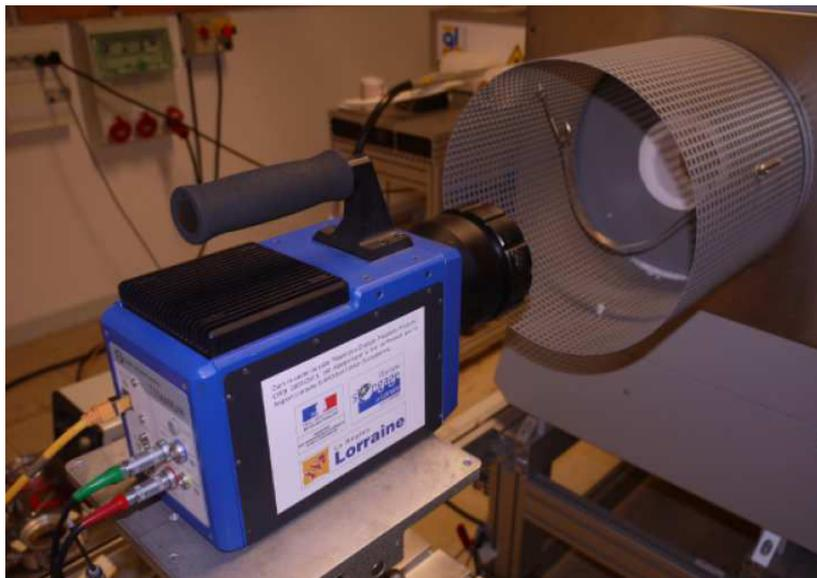
FIGURE 3.9 – Caméra infrarouge Cedip/Flir Titanium [122]
