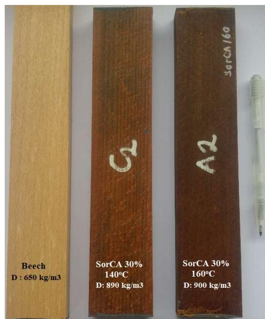
Figure 9 Beech and SorCA 30%-impregnated wood cured at 140 and 160°C
