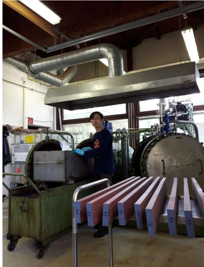
**Figure 35:** Vacuum-pressure impregnation chambers during up-scaling, Wood Biology and Wood Technology, Göttingen University, 2018
