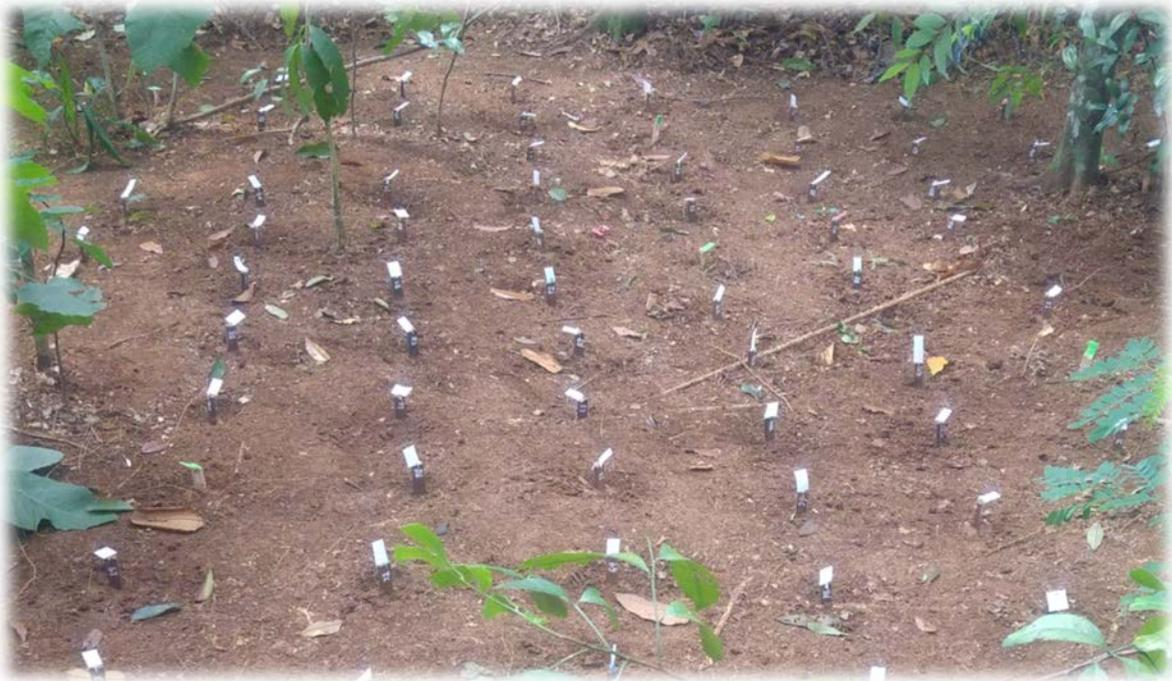
**Figure 1.** Samples position set during graveyard test
