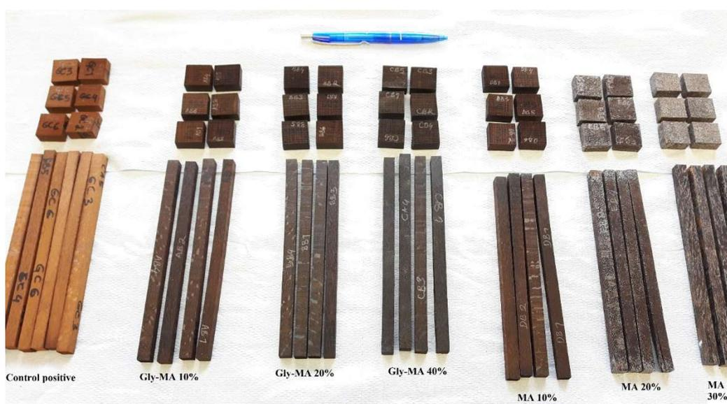
Figure 21 Additive-treated wood and wood control under HPS system at  $160^{\circ}\text{C}$
