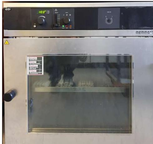
**Figure 33:** Oven heating (OHT) equipment, Wood Biology and Wood Technology, Göttingen University, 2018
