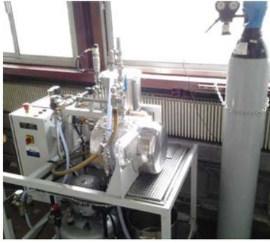
**Figure 1: Autoclave for vacuum-pressure impregnation and thermal treatment**
