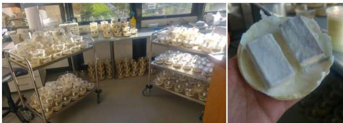
**Figure 37:** Decay test against *Coniophora puteana* (CP) and *Trametes versicolor* (TV), Wood biology and Wood Technology, Gottingen University, 2019
