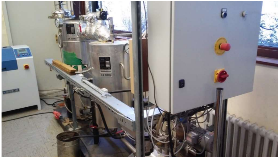
Figure 34: Autoclave for thermal wood modification, Wood Biology and Wood Technology, Göttingen University, 2018
