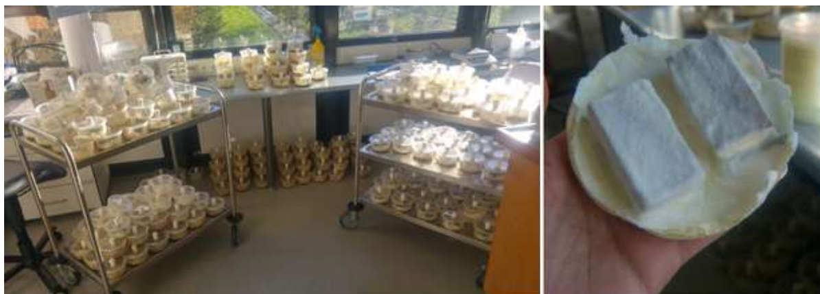
Figure 37: Decay test against Coniophora puteana (CP) and Trametes versicolor (TV), Wood biology and Wood Technology, Gottingen University, 2019
