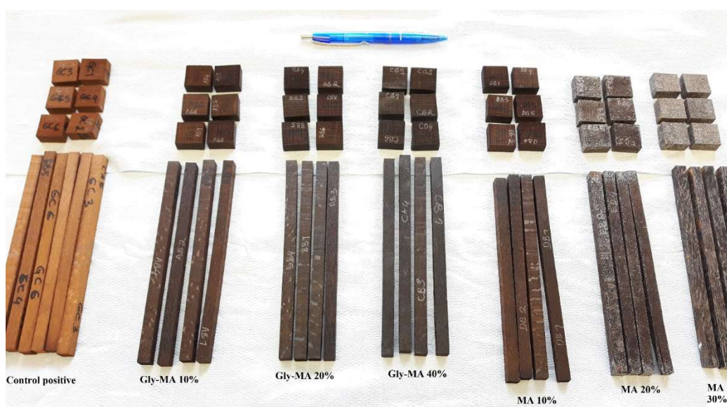
Figure 21 Additive-treated wood and wood control under HPS system at 160°C
