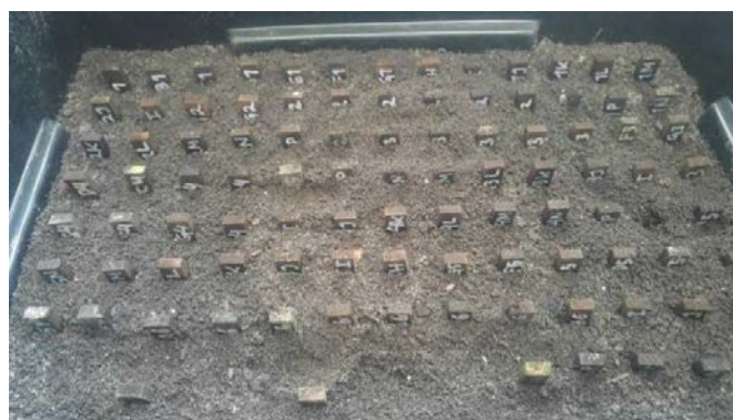
Figure 39: Samples set in soft-rotting micro fungi test, after 4 months period
