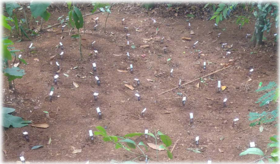
Figure 1. Samples position set during graveyard test
