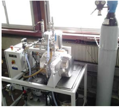
Figure 1: Autoclave for vacuum-pressure impregnation and thermal treatment
