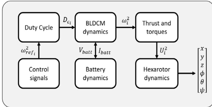
Figure 3.10: Interaction between propulsion system and hexarotor dynamics.
