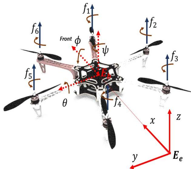
Figure 3.5: Reference frames of the UAV hexarotor.
