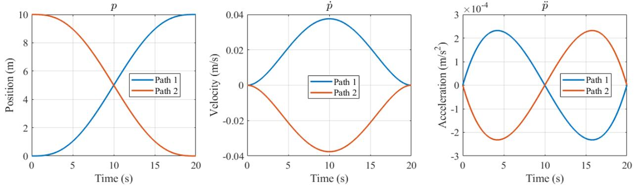
Figure 5.3: Example of path generation with polynomial function.
