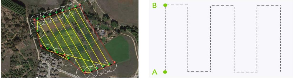
Figure 5.2: Example of crop irrigation path for multirotors.
