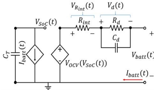
Figure 3.9: Electrical equivalent circuit of Li-Po battery.
