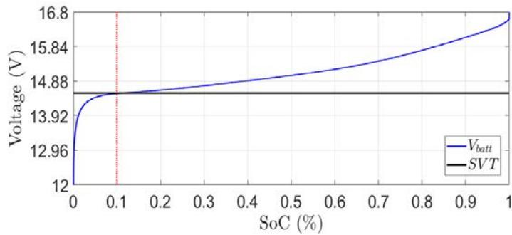
Figure 4.9: Safety Voltage Threshold of the Li-Po battery.
