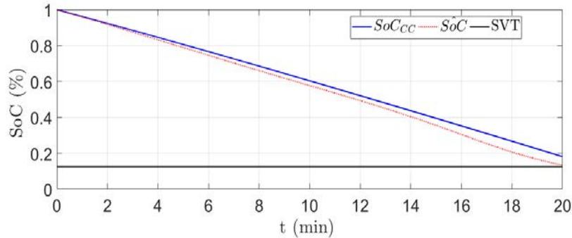
Figure 4.12: Comparison between  $SoC_{CC}$  and  $\hat{SoC}$ .
