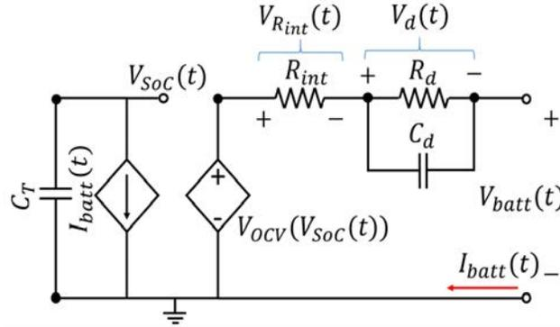
Figure 6.1: Equivalent Circuit Model of Li-Po battery.
