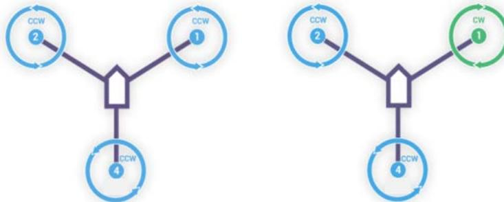
Figure 3.1: Trirotor flight configurations ([58]).
