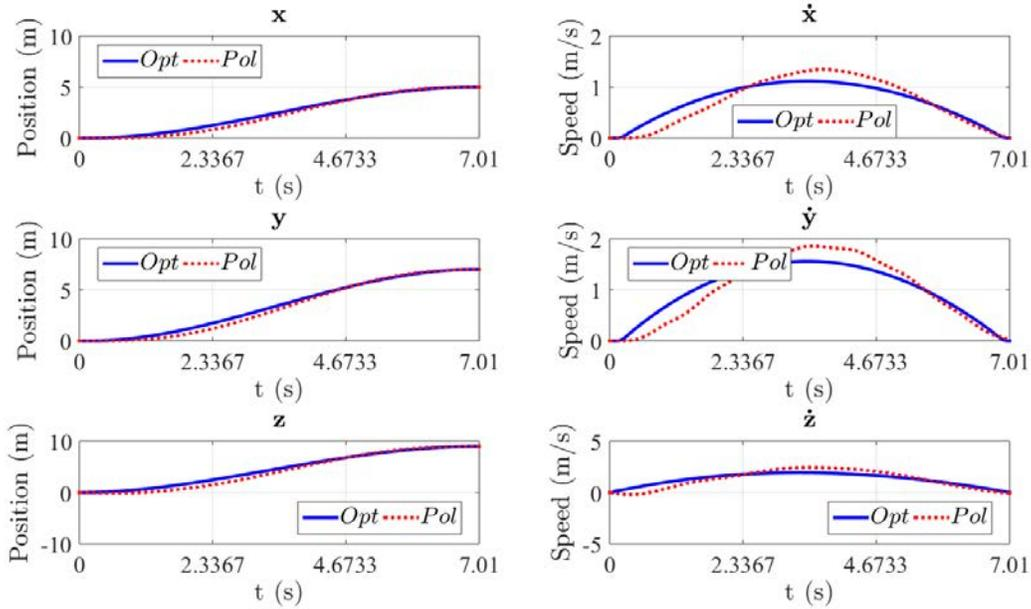
Figure 5.10: Case 1: Position and linear speed around  $x - y - z$  axis.
