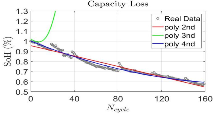
Figure 4.6: Fitting of capacity loss with polynomial functions.
