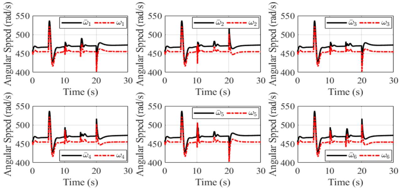
Figure 3.18: Angular speed of BLDCMs.
