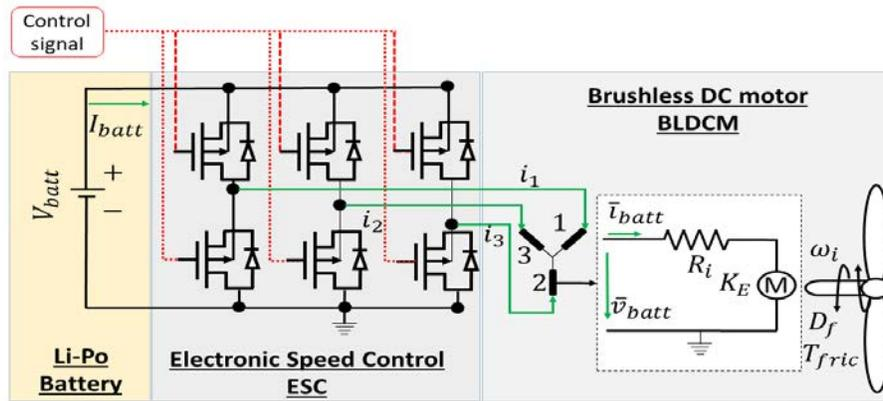
Figure 3.7: Connexion of Li-Po battery - ESC - BLDCM.
