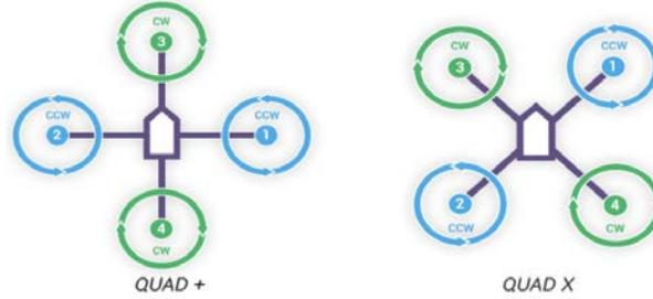
Figure 3.2: Quadrotor + and **X** flight configurations ([58]).
