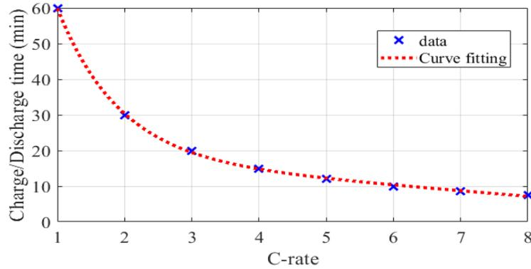
Figure 1.3: Relationship of C-rate and charge/discharge time.
