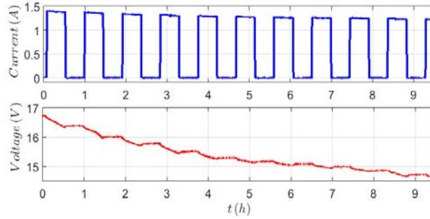
Figure 6.2: Discharge current profile and battery voltage.
