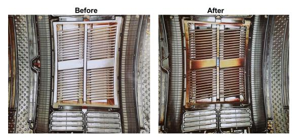
Figure A26: Q1 ICRF antenna before and after the WEST C3b campaign
