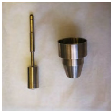
Figure 2.3 – Couette geometry: stator on the left and rotor on the right
