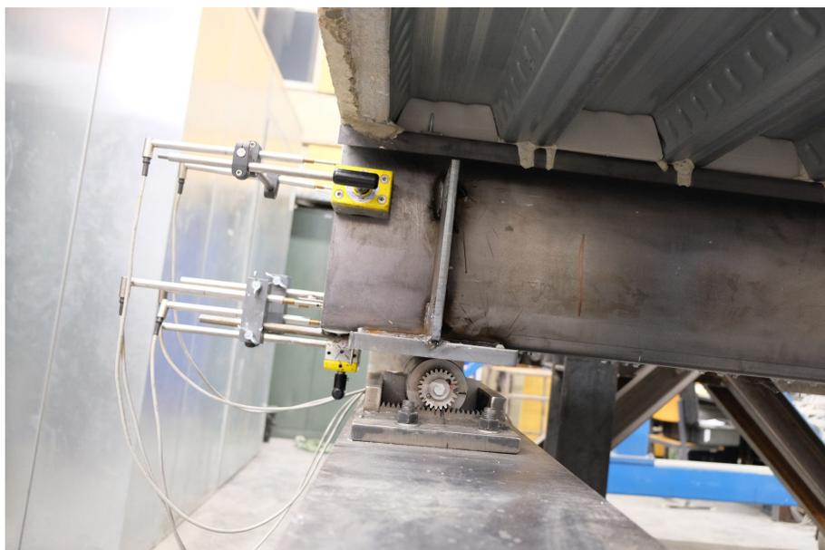
**Figure 6.17** – One roller support and the displacements sensors for the end-slip
