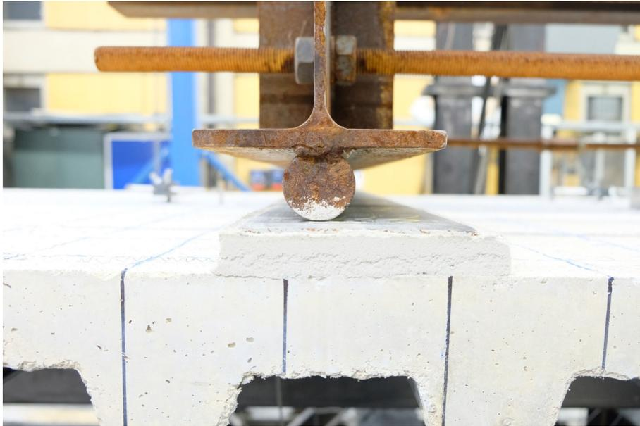
**Figure 6.19** – Detail of the loading introduction
