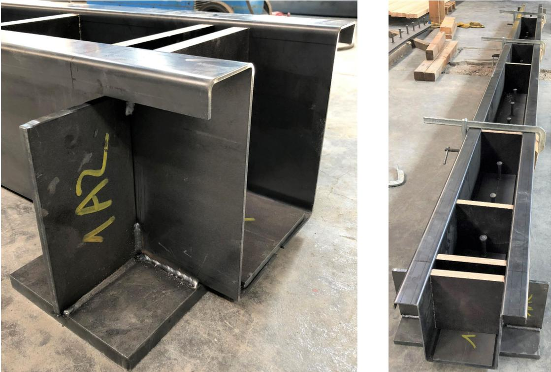
Figure 4.4 – Assembly of the supports and positioning of the side plates
