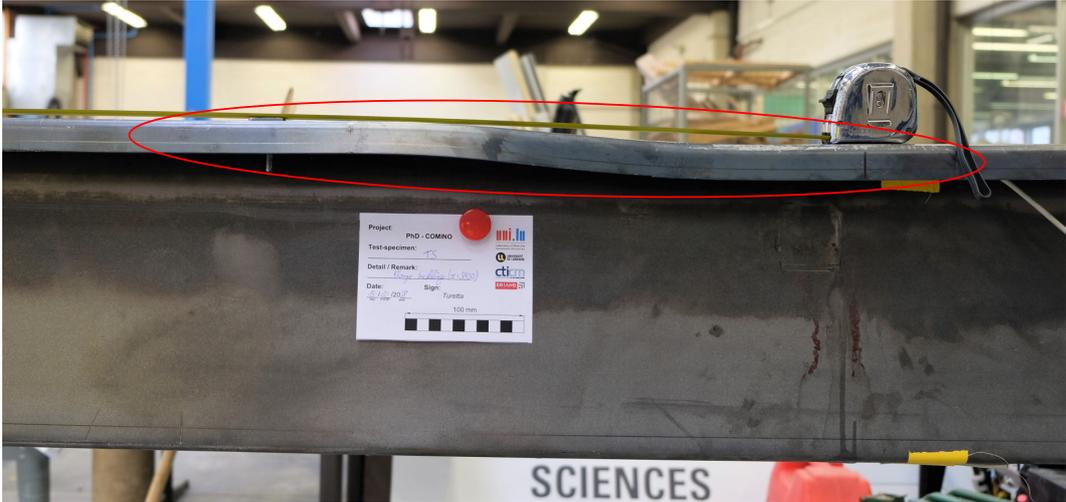
Figure 4.27 – Deformed shape in flange buckling after failure
