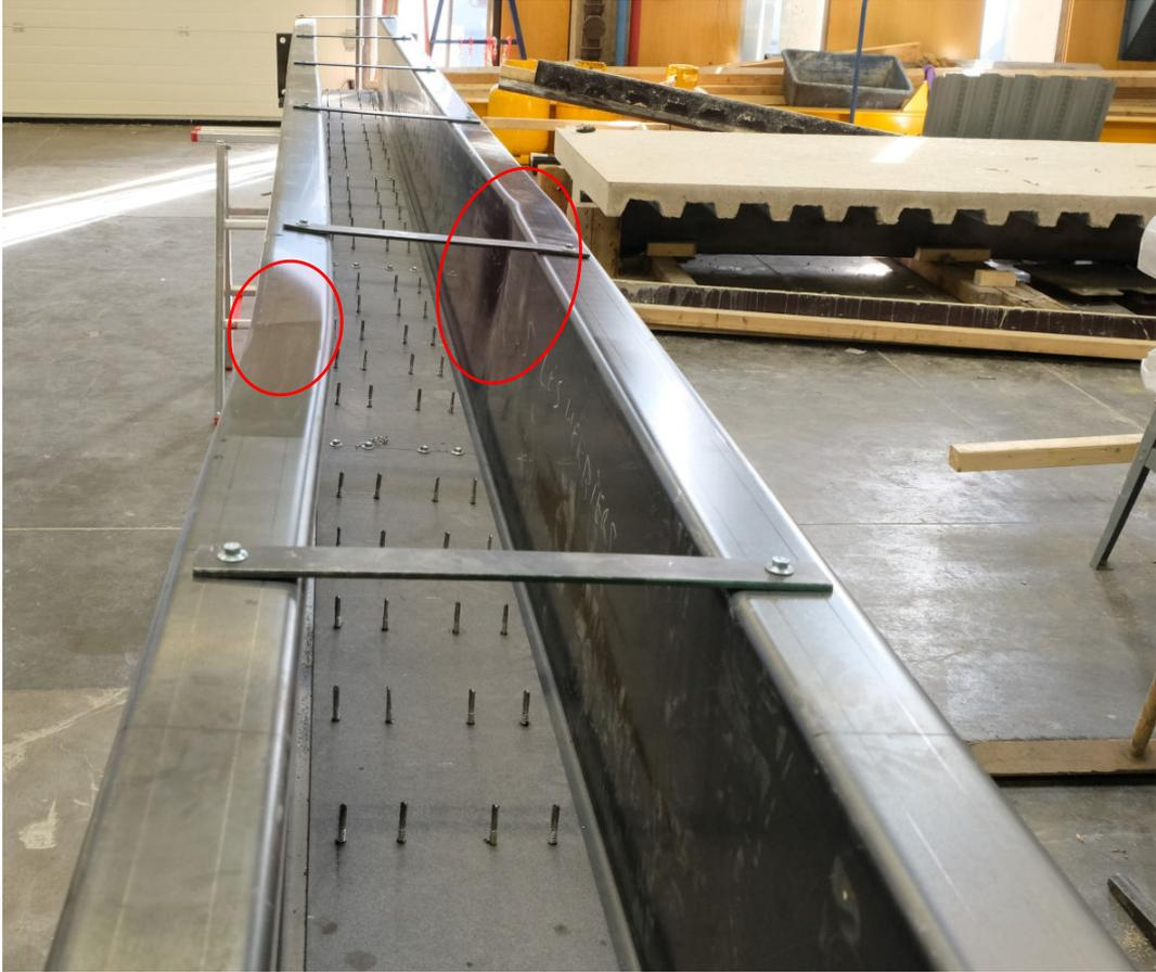
Figure 4.28 – Global residual deformed shape after the test
