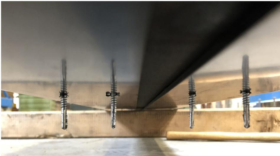
**Figure 4.5** – The self-drilling screws in the “wrong” direction before being cut
