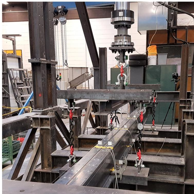
**Figure 4.14** – The beam specimen reversed and placed in the test frame
