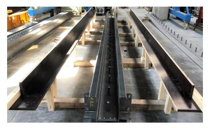
Figure 6.3 – The steel beam placed in the formwork
