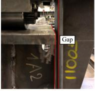
(b) Gap between beam and guidance
