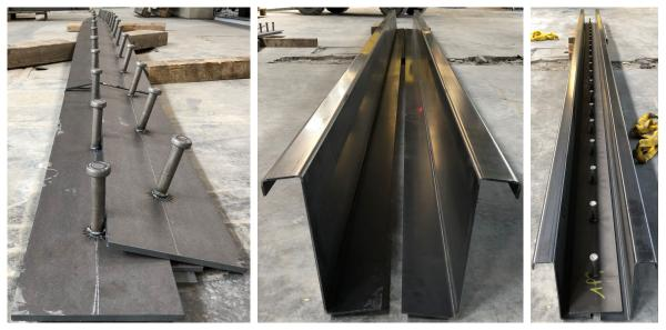
Figure 4.3 – Preliminary assembly of the steel beam
