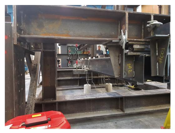
Figure 4.16 – The U-shaped beam reversed and placed in the test frame
