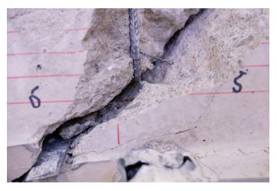
Figure 6.44 – Failure of the stirrup in the major crack
