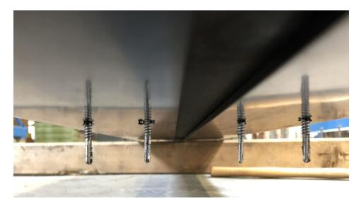
Figure 4.5 – The self-drilling screws in the "wrong" direction before being cut
