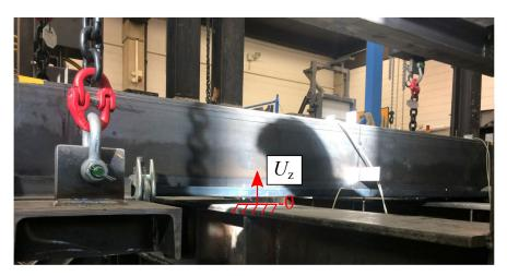
Figure 4.22 – The vertical deflection of the beam at the begin of the test
