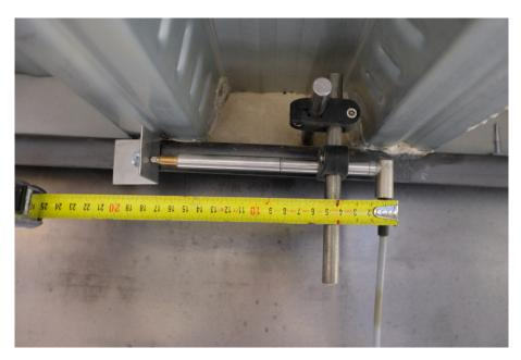
Figure 6.24 – Displacement sensor for the slip under one point load (DISP25)
