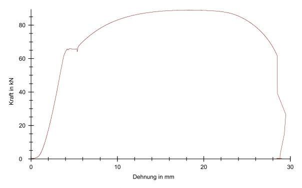
Figure A.10 – Tensile test curve of C1
