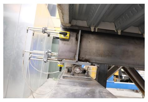
Figure 6.17 - One roller support and the displacements sensors for the end-slip
