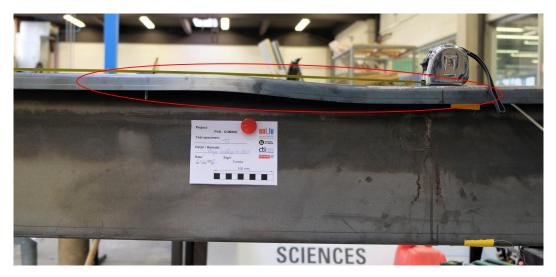
Figure 4.27 – Deformed shape in flange buckling after failure
