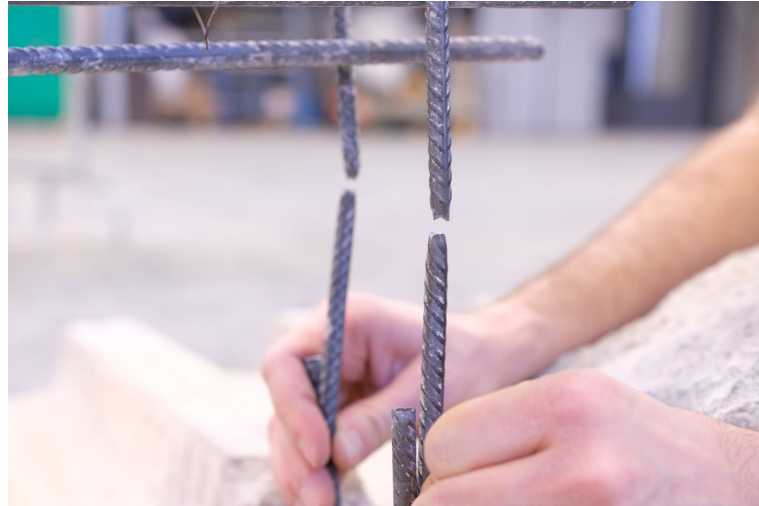
Figure 6.45 – Failure on both sides of the steel stirrup
