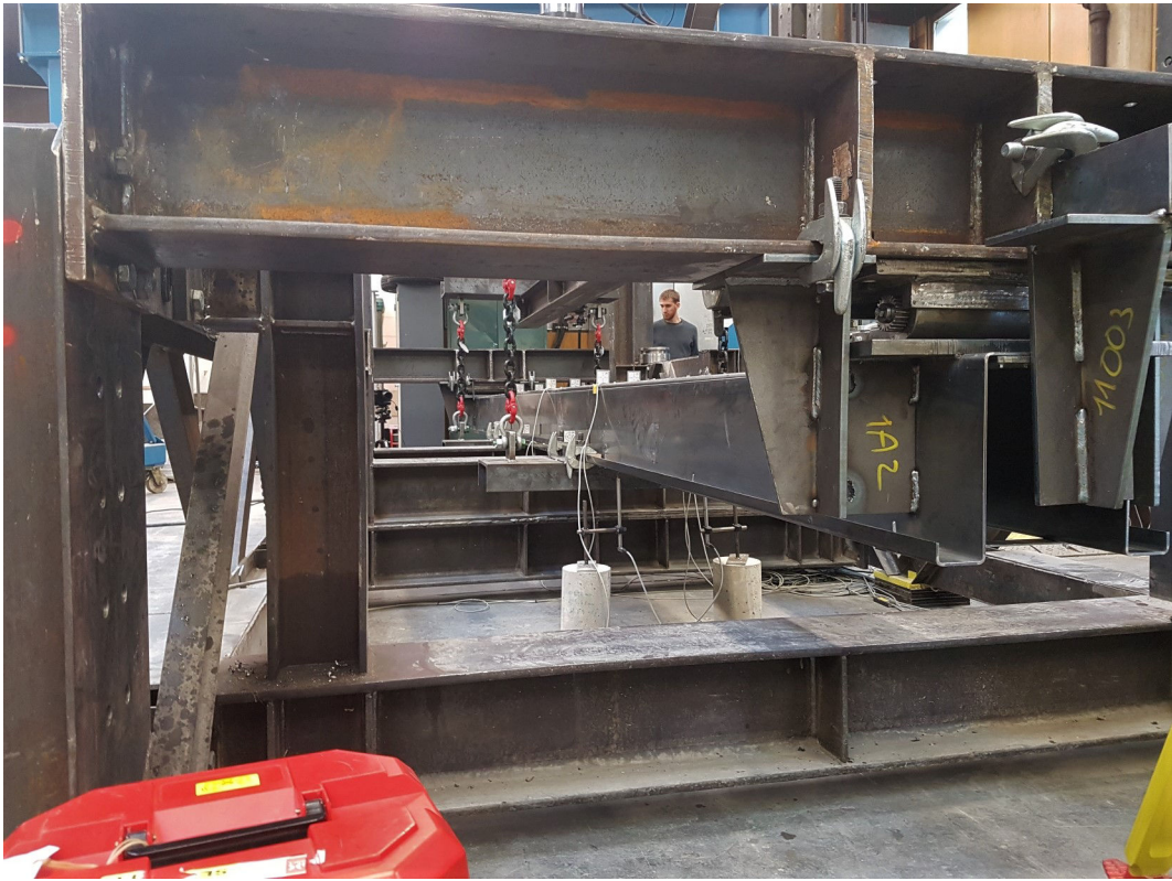
Figure 4.16 – The U-shaped beam reversed and placed in the test frame
