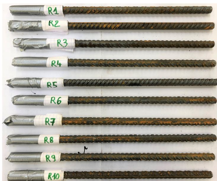
Figure 6.2 – Tensile specimens of the rebars (R1 to R10)
