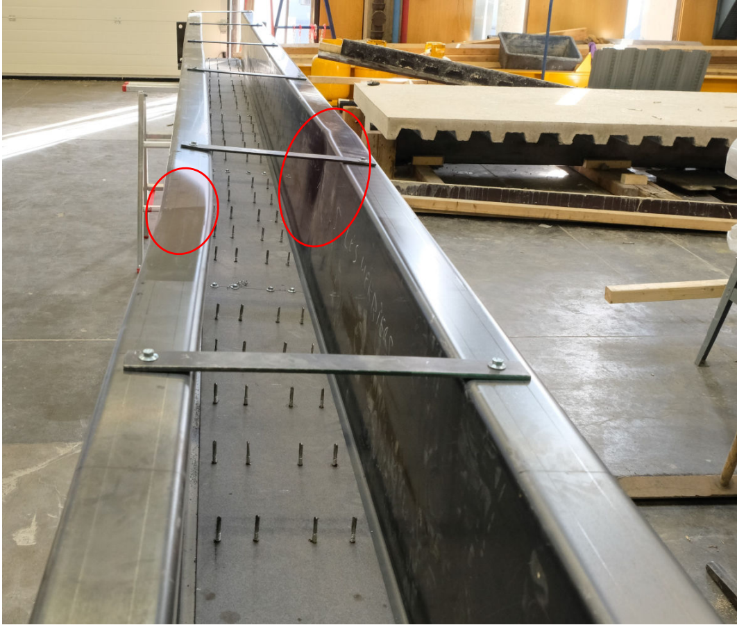
Figure 4.28 – Global residual deformed shape after the test
