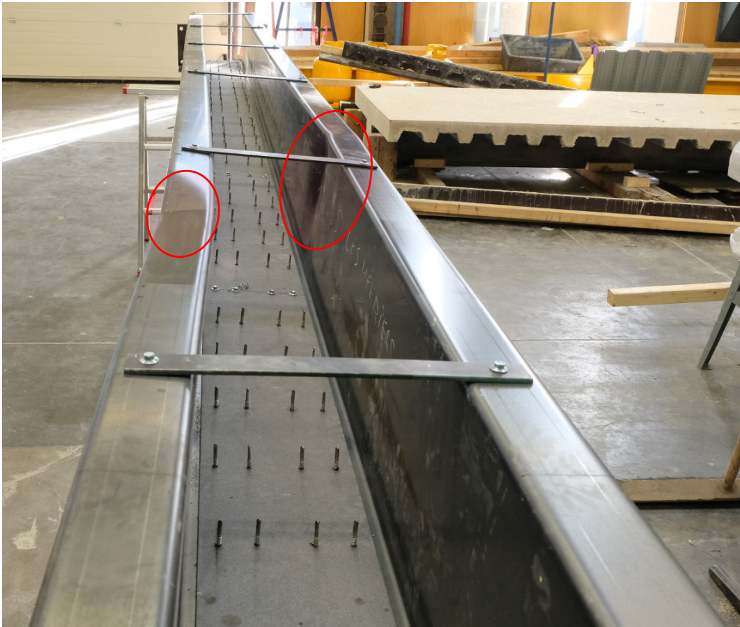
Figure 4.28 – Global residual deformed shape after the test
