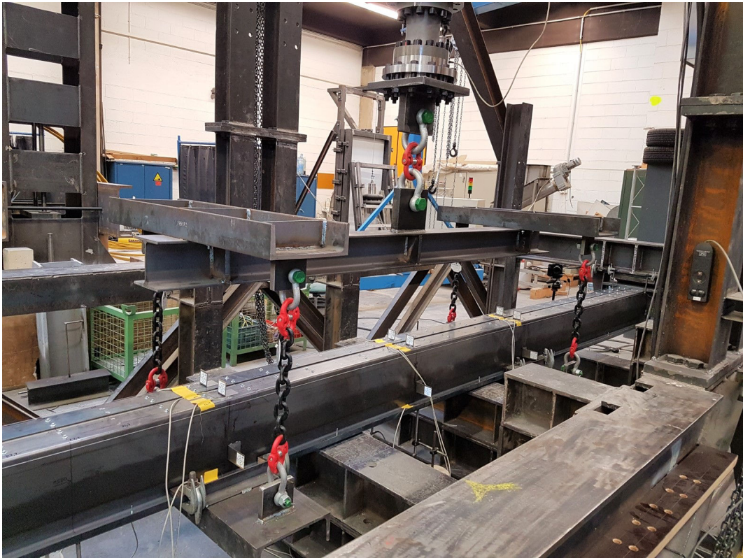
Figure 4.15 – The loading system – side view
