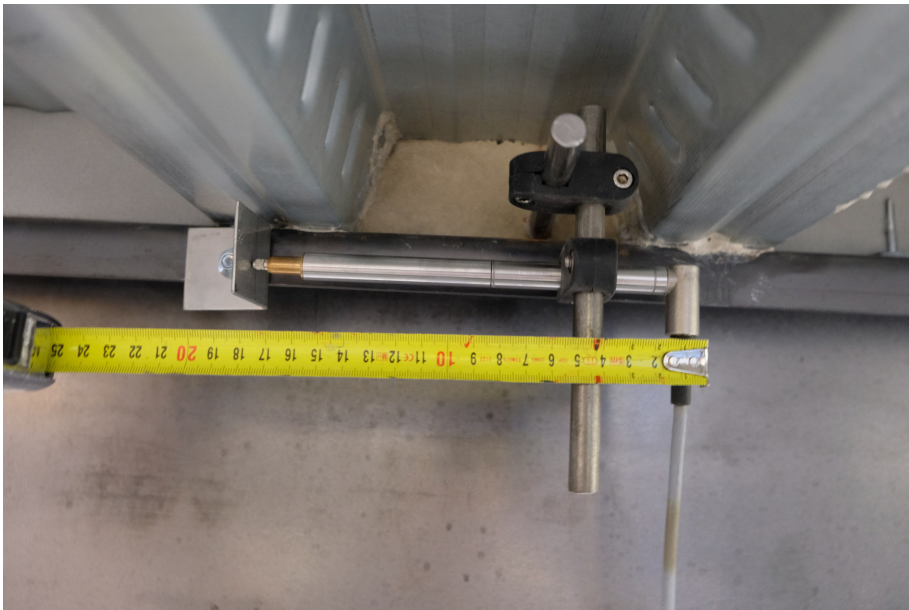
Figure 6.24 – Displacement sensor for the slip under one point load (DISP25)
