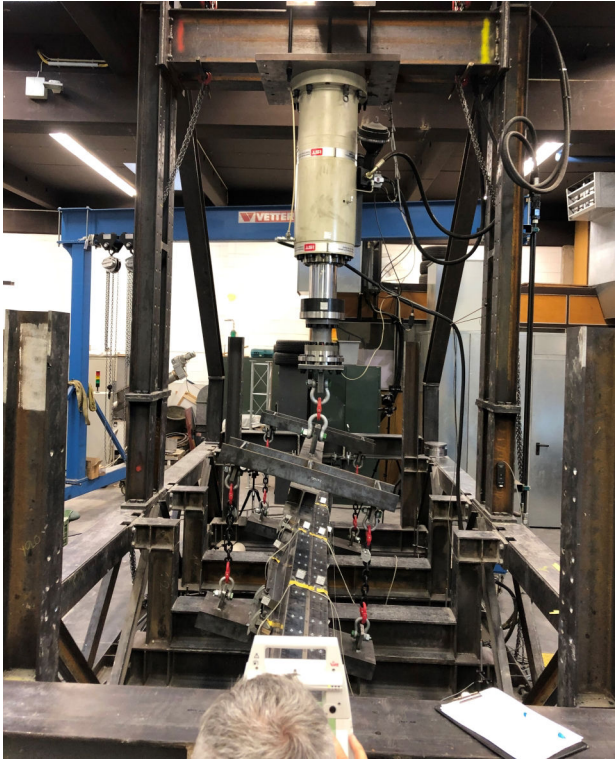
Figure 4.24 – LTB instability followed with the targets
