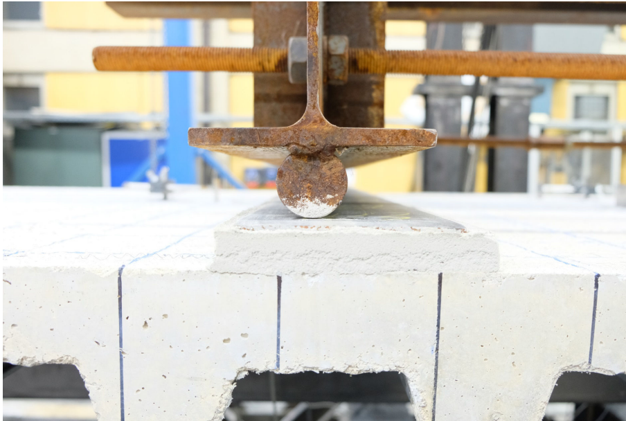
Figure 6.19 – Detail of the loading introduction
