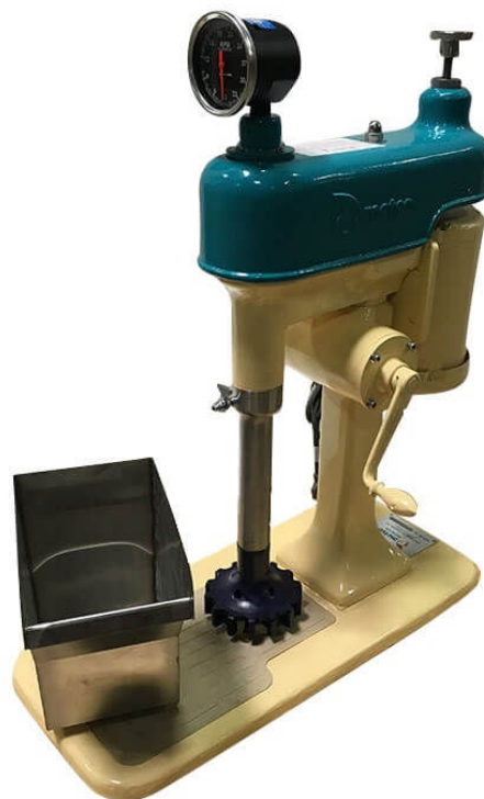
Fig. 3.5 – Denver type flotation machine, Metso D-12.
