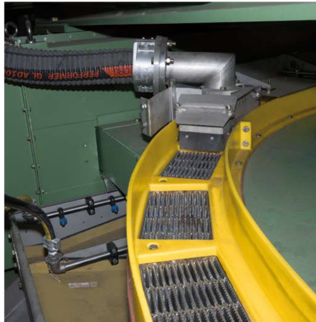
Fig. 2.7 – Circular structure of a high-intensity magnetic separator type Jones from MBE ® .
