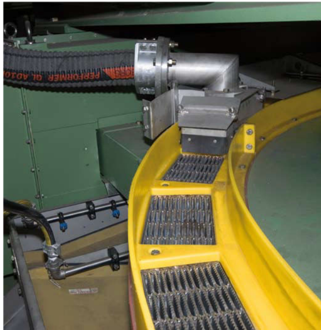
Fig. 2.7 – Circular structure of a high-intensity magnetic separator type Jones from MBE ® .
