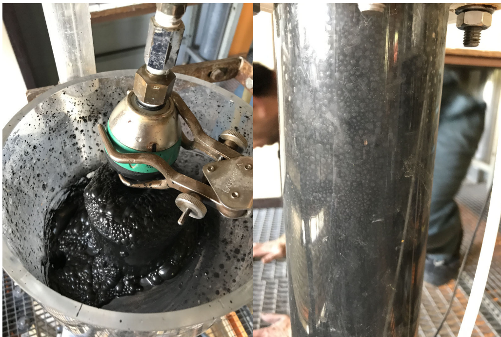
Fig. 7.5 – Column flotation froth view on top ( left ) and lateral ( right ).
