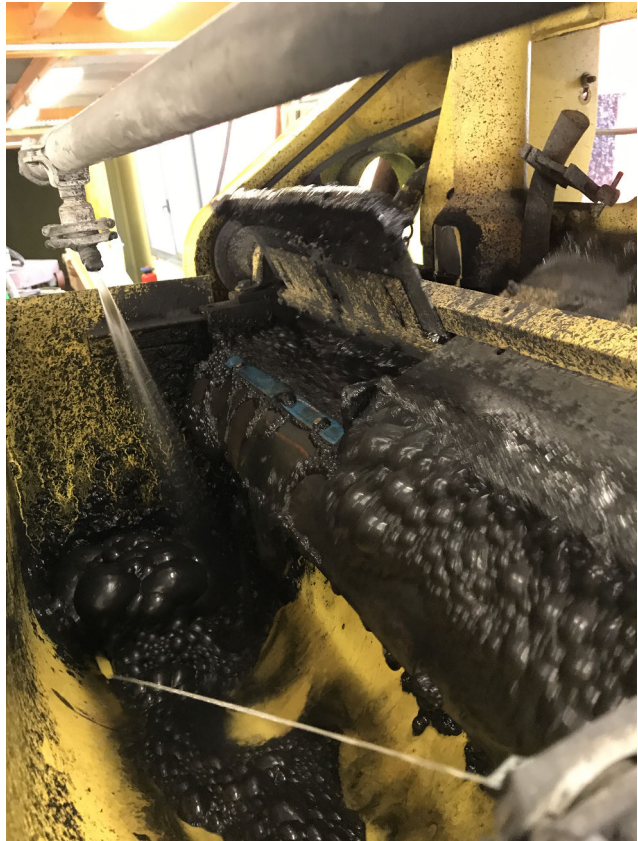
Fig. 7.3 – Froth of the rougher stage of the pilot flotation test.
