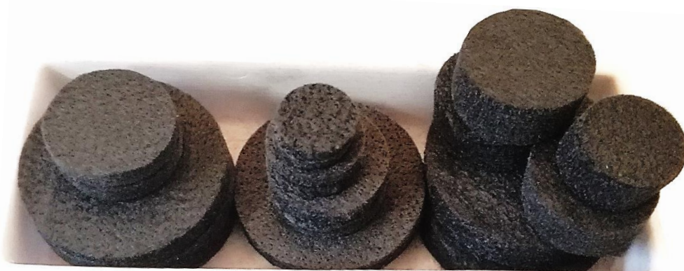
Figure I/3-2 Needle-punched carbon felt samples (carbonised to graphitised, from left to right).
