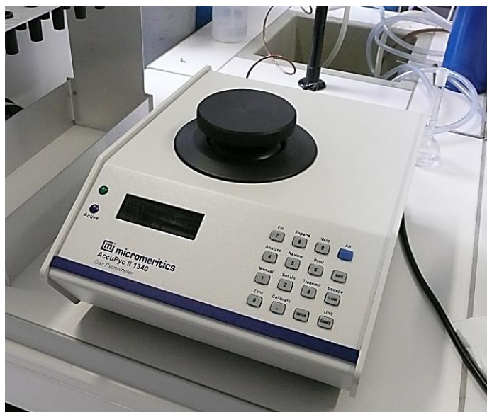
Figure II/2-1 Helium pycnometer AccuPyc II 1340 (Micromeritics, USA) automatic apparatus.
