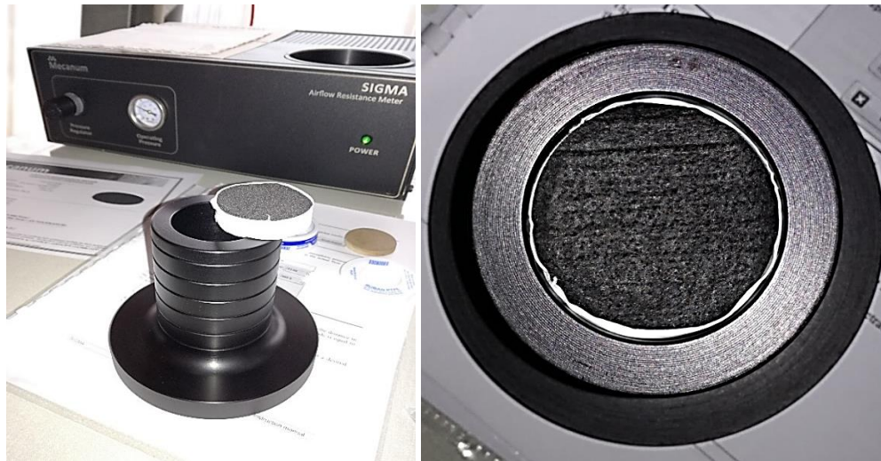
Figure II/2-7 Left - prepared sample and sample holder for airflow resistance measurement; right - top view of sample holder with installed sample.
