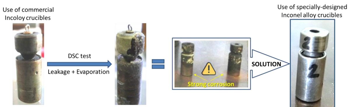
Figure IV/3-22 Failure to use Incoloy alloy crucibles to perform DSC tests, and identified problems and solutions considered for future examinations (modified after project Pc2TES ANR -16-CE06-0012-0 meeting presentation by F. Achchaq)
