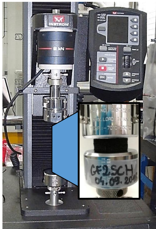
Figure II/2-2 Measurement of carbon non-woven material's thickness by use of an Instron 5944 universal testing machine.
