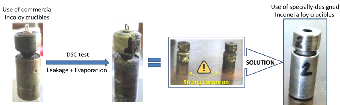
Figure IV/3-22 Failure to use Incoloy alloy crucibles to perform DSC tests, and identified problems and solutions considered for future examinations (modified after project Pc2TES ANR -16-CE06-0012-0 meeting presentation by F. Achchaq)
