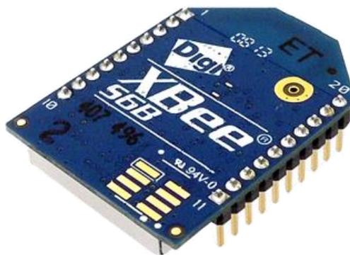
**Figure 68.** Module XBee.
