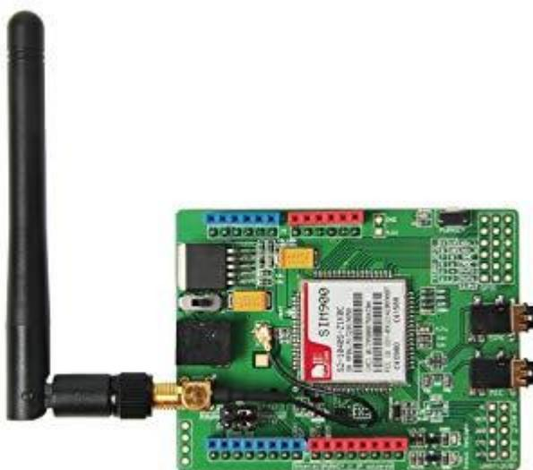
**Figure 70.** Module GSM SIM900
