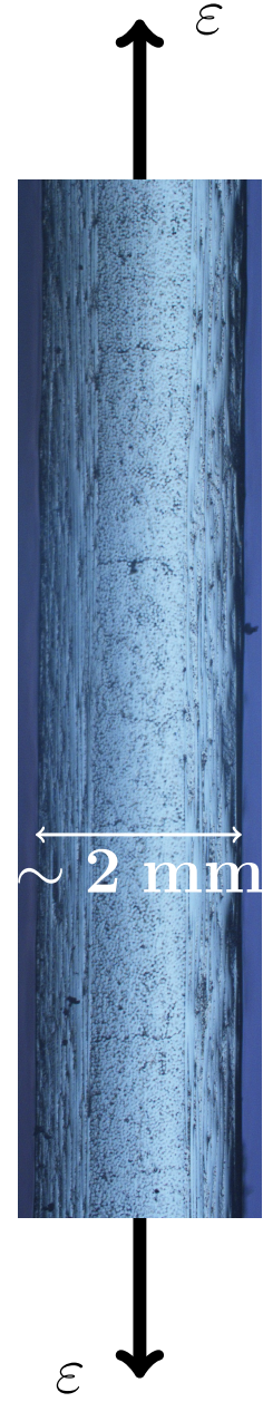
(b) Edge view, optical microscope, [0, 90]_S . The horizontal black lines in the central 90^\circ layer are transverse cracks.
