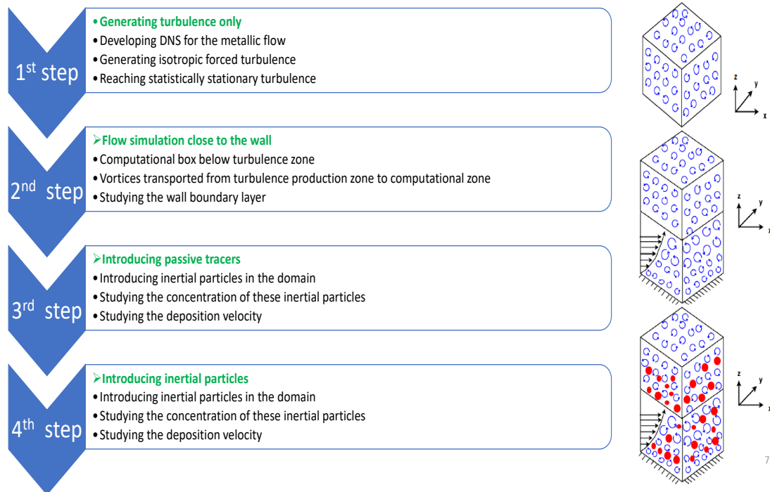
Figure 1.19 – Schematic showing the numerical methodology followed in the thesis
