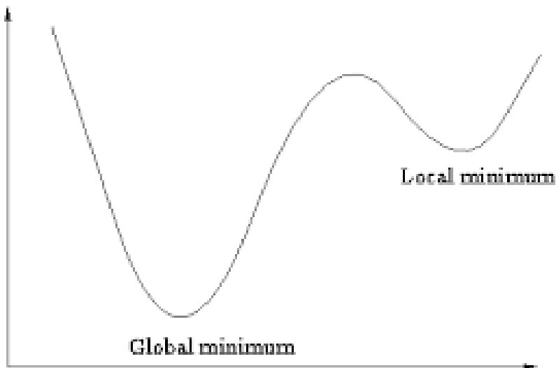
Figure 5.15: Local and global minimum of a non-linear function
