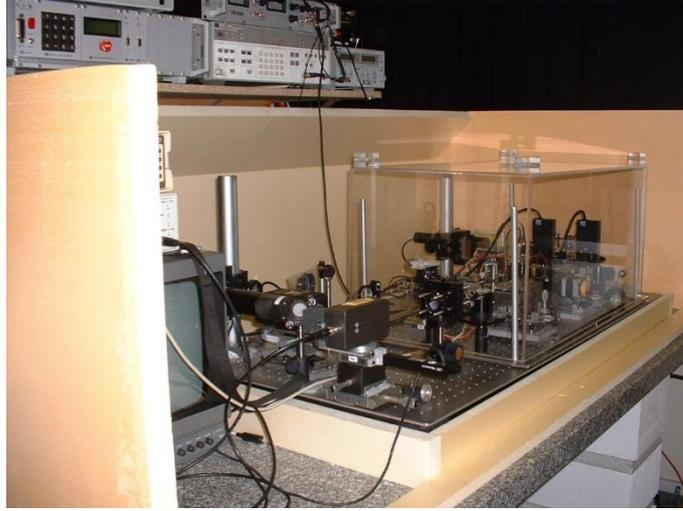
Figure 3.1.1.2.2: Mach-Zehnder interferometric setup.
