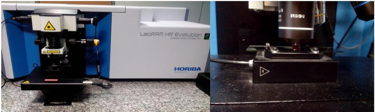
Figure 2.2.1.1: LabRAM HR Evolution Raman spectrometer.
